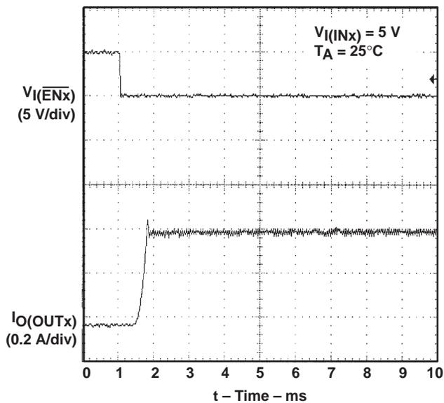
Figure 6. TPS2047, Short-Circuit Current, Device Enabled into Short
