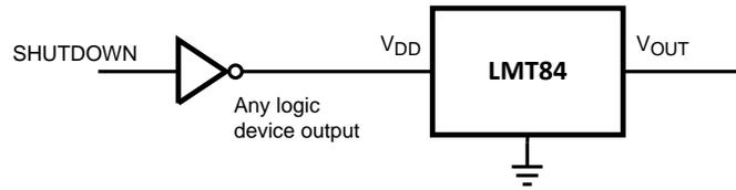
Figure 15. Simple Shutdown Connection of the LMT84
