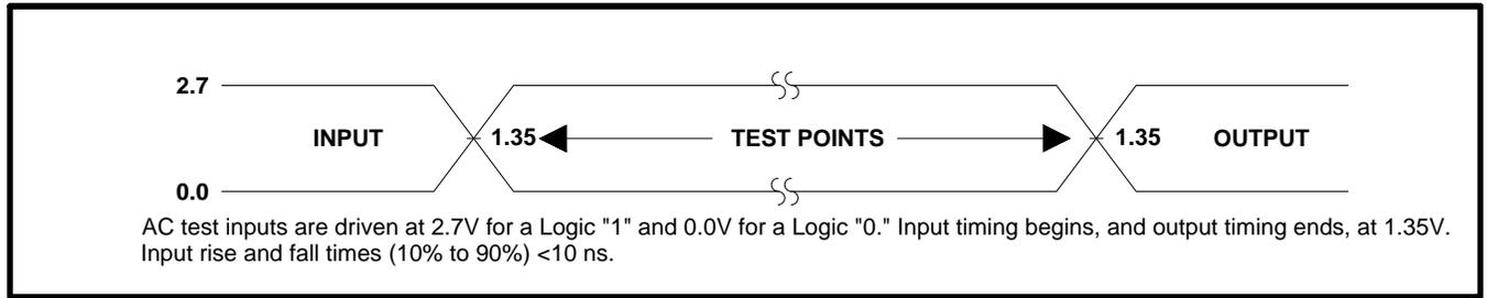
Figure 11. Transient Input/Output Reference Waveform for  $V_{CC}=2.7V-3.6V$
