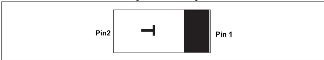
Note: Product marking may be rotated by multiples of 180° for assembly plant differentiation. In no case should this product marking be used to orient the component for its placement on a PCB. Only pin 1 mark is to be used for this purpose.
