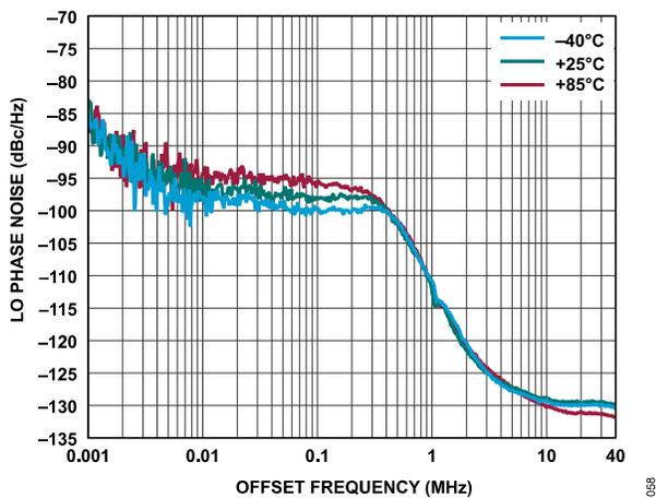
Figure 57. LO Phase Noise vs. Offset Frequency at 18.6 GHz and at Various Temperatures, CP\_CURRENT = 4 and SI\_VCO\_CORE = 1
