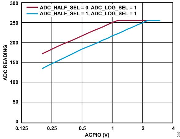
Figure 49. ADC Reading vs. AGPIO for ADC\_LOG\_SEL = 1
