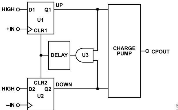
Figure 87. PFD and Charge Pump Simplified Schematic
