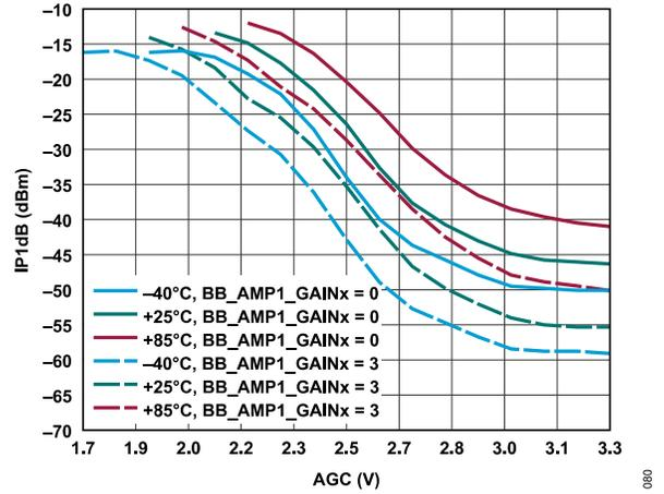
Figure 79. IP1dB vs. AGC, LO = 21 GHz Various Temperatures
