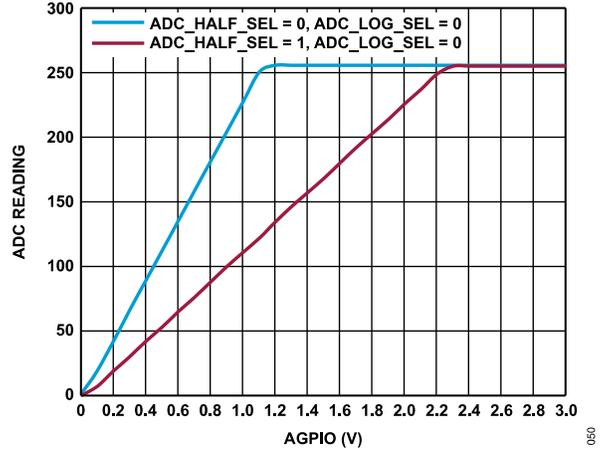
Figure 50. ADC Reading vs. AGPIO for ADC\_LOG\_SEL = 0
