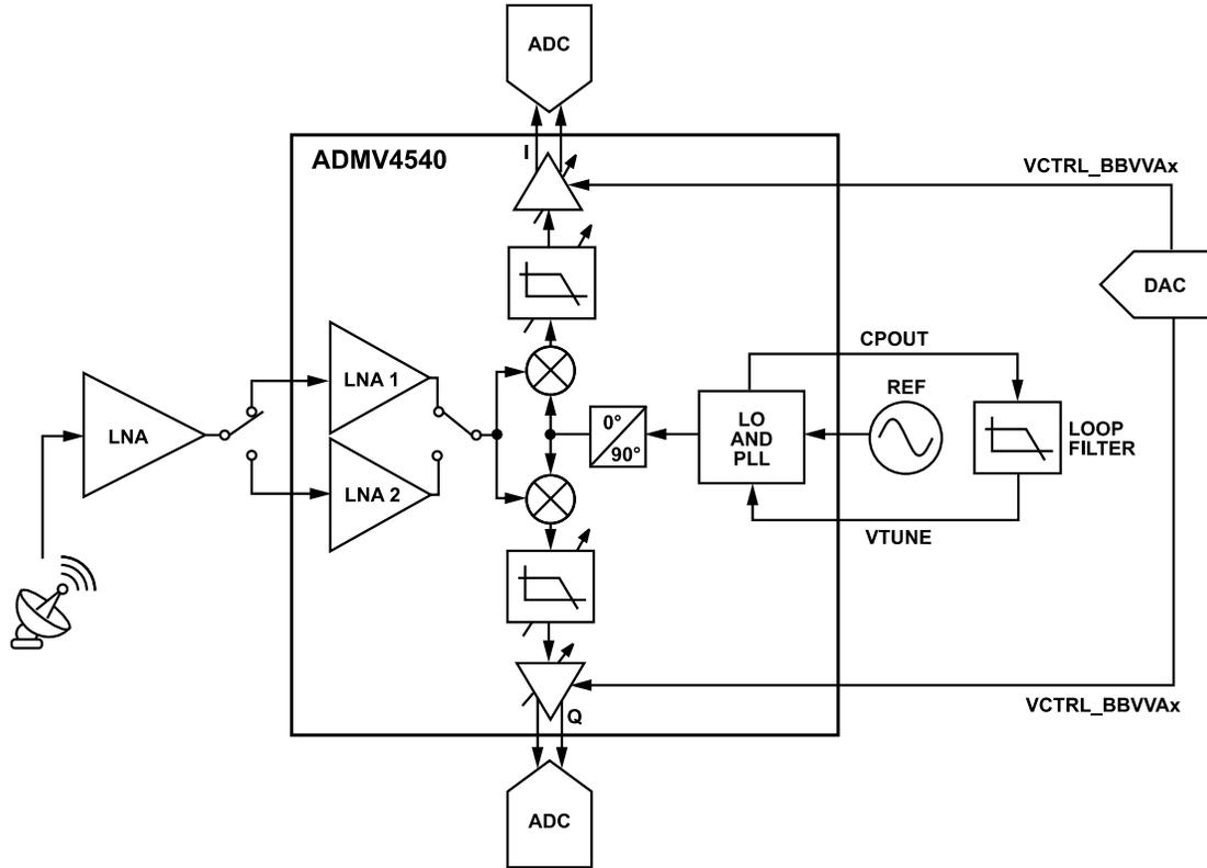
Figure 88. System Block Diagram of the ADMV4540
