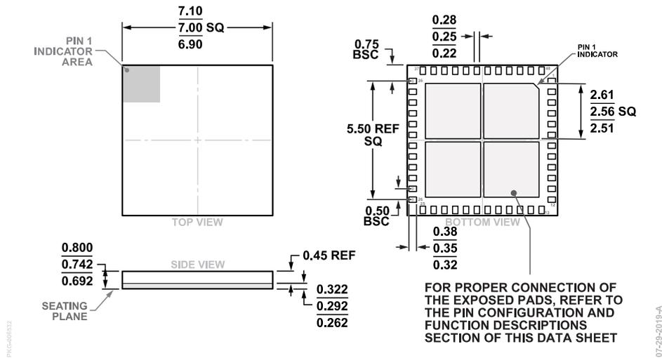
Figure 89. 48-Terminal Land Grid Array [LGA]
