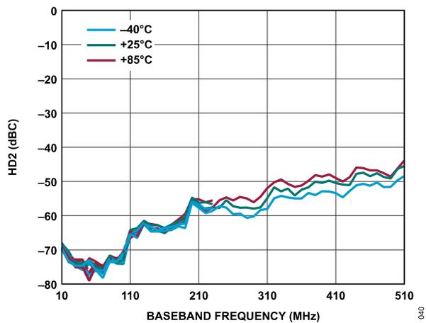
Figure 40. Harmonic Distortion 2 (HD2) vs. Baseband Frequency at 20 dB Gain (Maximum Input Power) and at Various Temperatures
