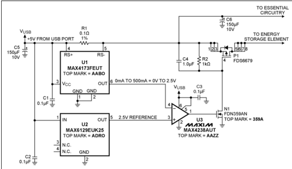
Figure 2. This circuit continuously monitors the total current drawn from the USB port, and dynamically adjusts the storage-element current as required to avoid exceeding the port's maximum output capability.
