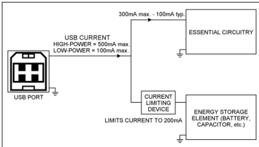
Figure 1. In this typical method for drawing power from a USB port, the storage-element current is limited to a fixed value that is less than optimal.
