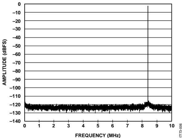
Figure 6. Single-Tone FFT with  $f_{IN} = 8.4$  MHz
