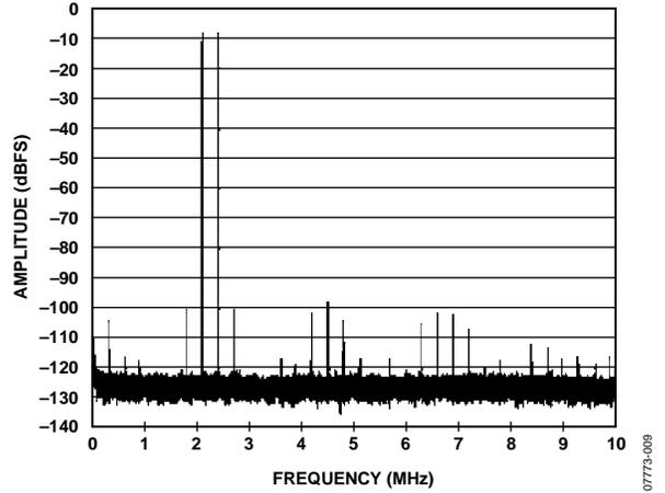
Figure 7. Two-Tone FFT with  $f_{IN1} = 2.1$  MHz,  $f_{IN2} = 2.4$  MHz
