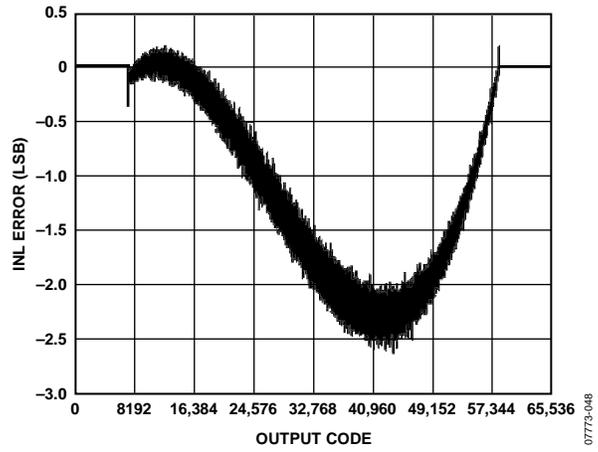
Figure 19. INL with  $f_{IN} = 2.4 \text{ MHz}$
