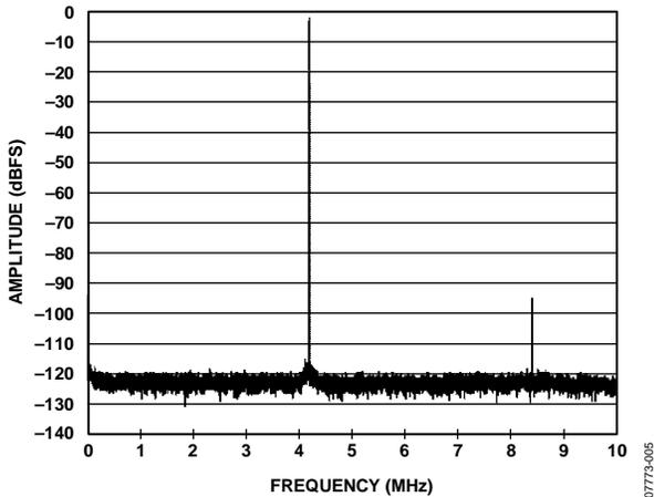
Figure 5. Single-Tone FFT with  $f_{IN} = 4.2$  MHz
