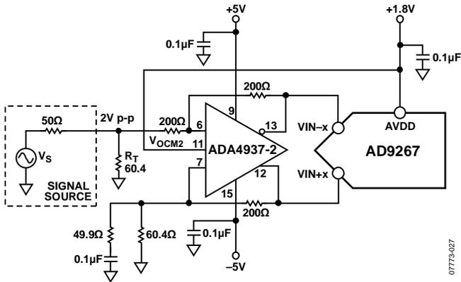
Figure 33. Differential Input Configuration Using the ADA4937-2
