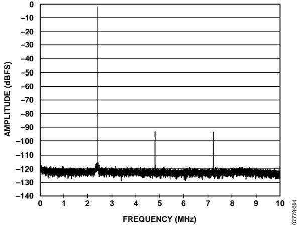
Figure 4. Single-Tone FFT with  $f_{IN} = 2.4$  MHz
