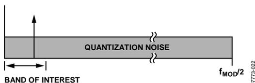
Figure 28. Quantization Noise
