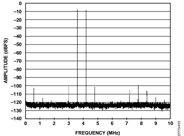
Figure 8. Two-Tone FFT with  $f_{IN1} = 3.6$  MHz,  $f_{IN2} = 4.2$  MHz
