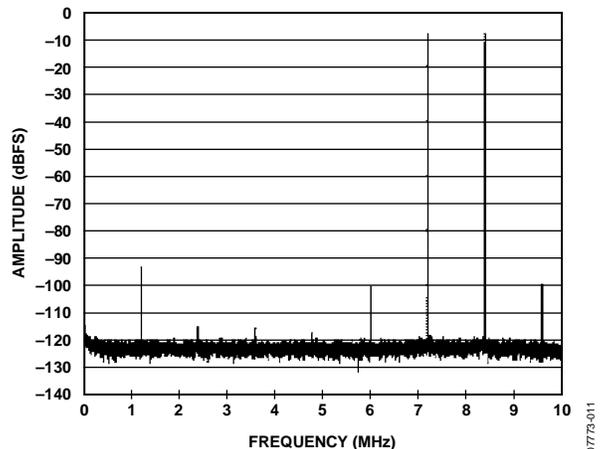
Figure 9. Two-Tone FFT with  $f_{IN1} = 7.2$  MHz,  $f_{IN2} = 8.4$  MHz
