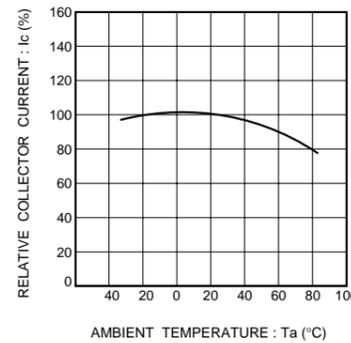
Fig.6 Relative output vs. ambient temperature
