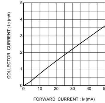
Fig.7 Collector current vs. forward current
