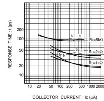
Fig.8 Response time vs. collector current
