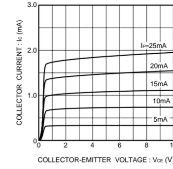
Fig.10 Output characteristics
