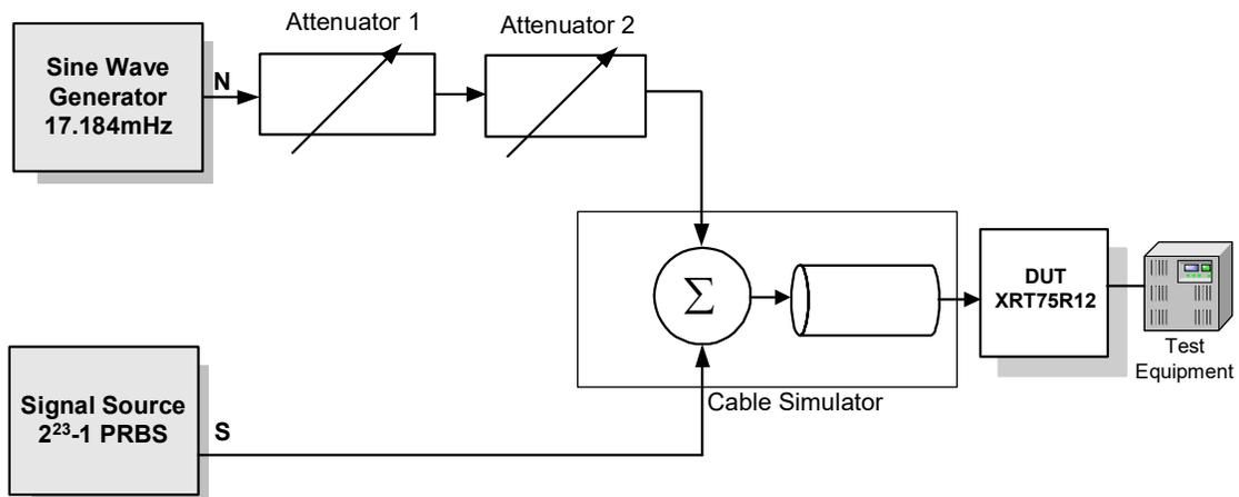
**Figure 10:** Interference Margin Test Set Up for E3
