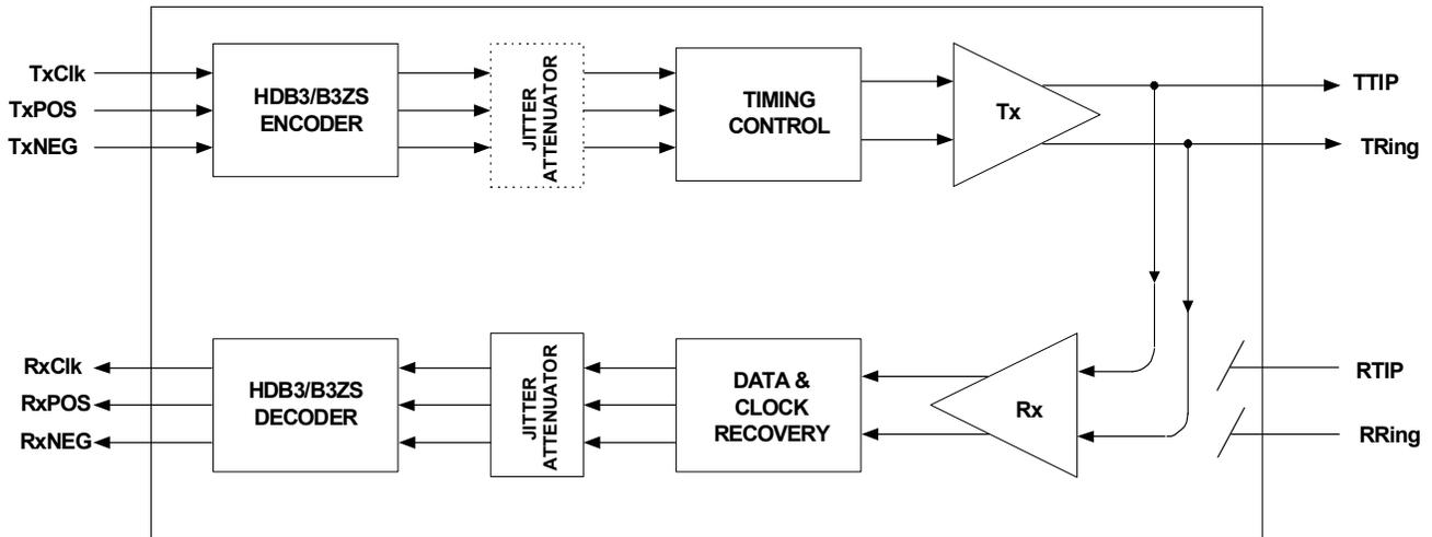
**Figure 29: Analog Loopback**
