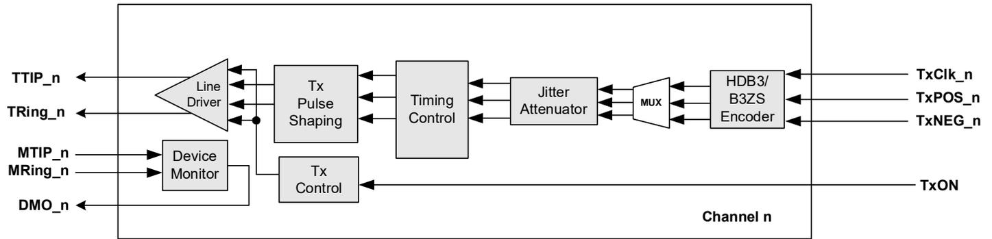
Figure 12: Transmit Path Block Diagram
