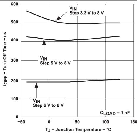
Figure 7. Turnoff Time to V<sub>GATE</sub> = 6.9 V vs Junction Temperature
