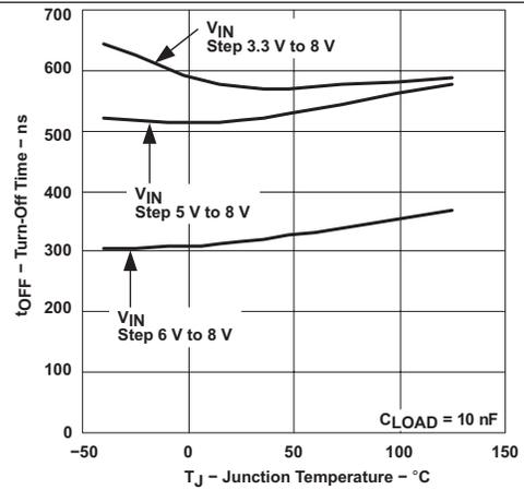
Figure 8. Turnoff Time to V<sub>GATE</sub> = 6.9 V vs Junction Temperature
