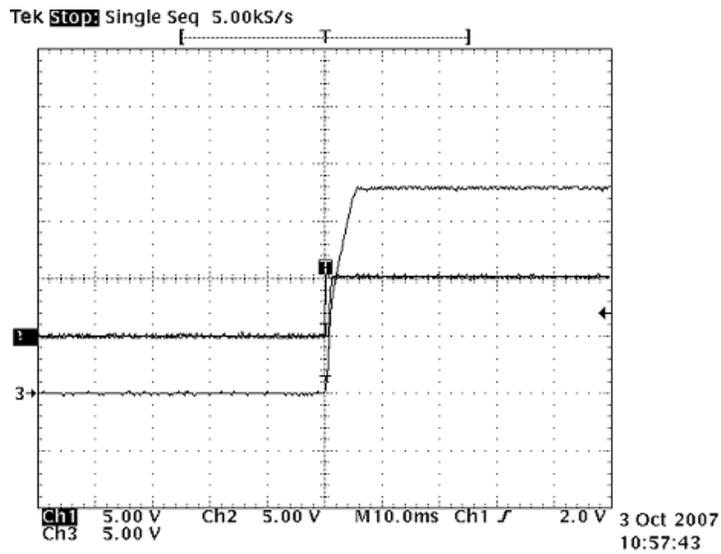
Figure 18. Circuit Start-Up With  $V_{IN} = 5\text{ V}$
