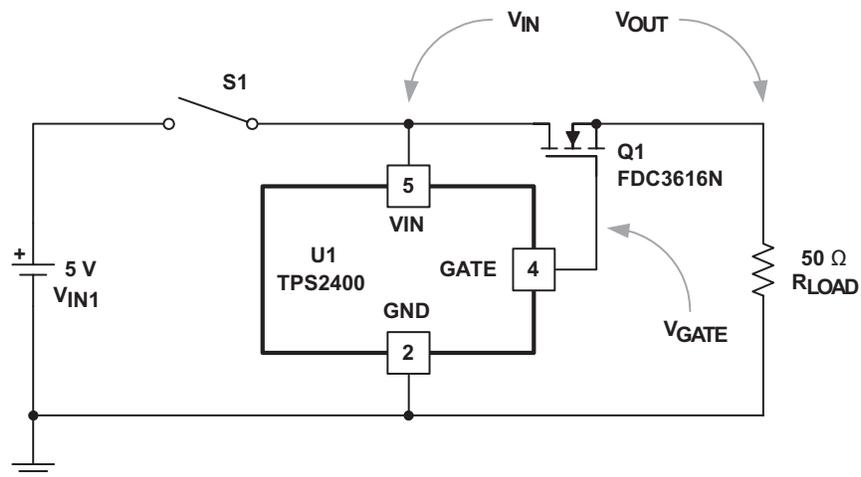
Figure 10. Output Turnon Response Test Circuit
