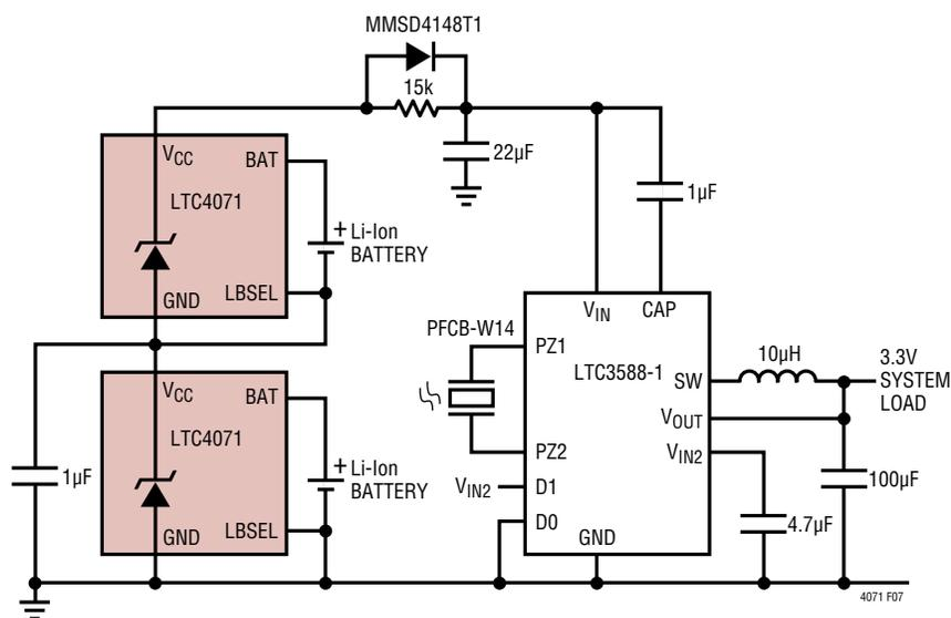
Figure 7. Piezoelectric Energy Harvester with Battery Backup
