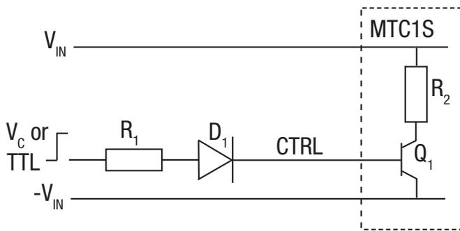
$D_1$  (e.g. 1N4001) is necessary for correct operation of the MTC1 when the control signal is LOW. The recommended drive current  $I_b$  to shut down the MTC1 is 6mA to 15mA. The value of  $R_1$  can be derived as follows:
