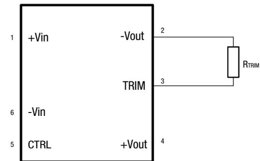
$$3.3V_{out} R_{TRIM} = \frac{14k \times V_{out} - 52.3k}{3.32 - V_{out}}$$
