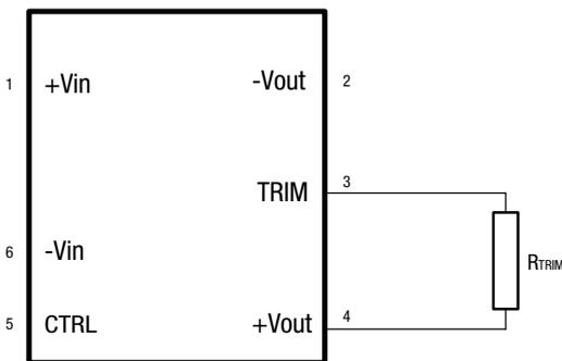
$$3.3V_{out} R_{TRIM} = \frac{18.64k \times V_{out} - 52.3k}{3.32 - V_{out}}$$
