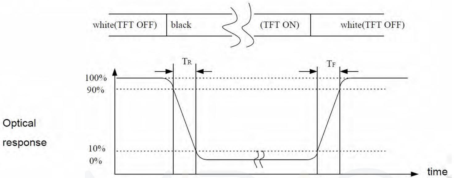
**Note (4)** Definition of optical measurement setup
