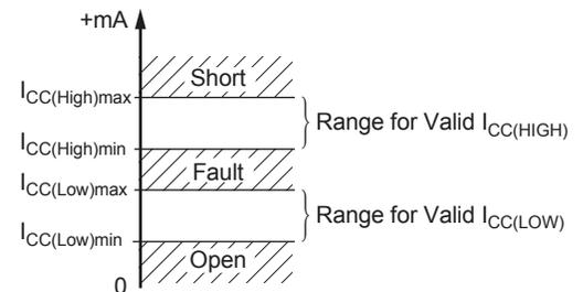
Figure 8: Diagnostic Characteristics of Supply Current Values
