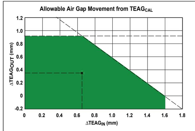
The colored area in the chart above shows the region of allowable air gap movement within which the sensor will continue output switching. The output duty cycle is wholly dependent on the target's magnetic signature across the air gap range of movement, and may not always be within specification throughout the entire operating region (to  $AG_{(OPmax)}$ ).
