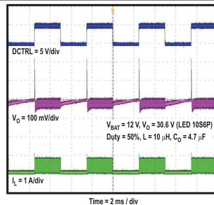
Figure 20. WLED Driver Output Ripple at PWM Dimming
