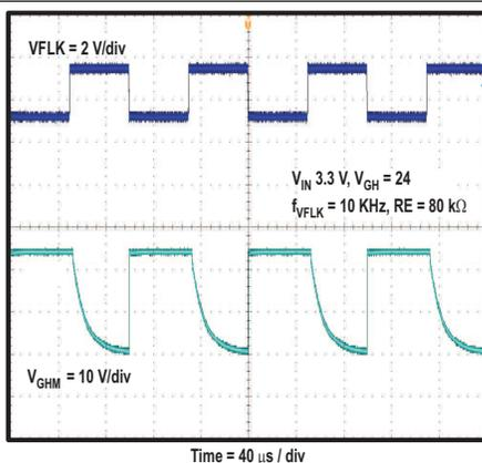
Figure 15. Gate Voltage Shaping
