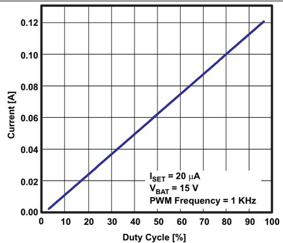
Figure 24. WLED Driver PWM Dimming Linearity 1 kHz
