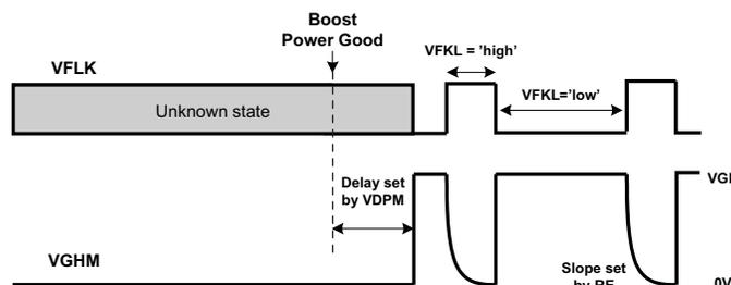
Figure 30. Gate Voltage Shaping Timing
