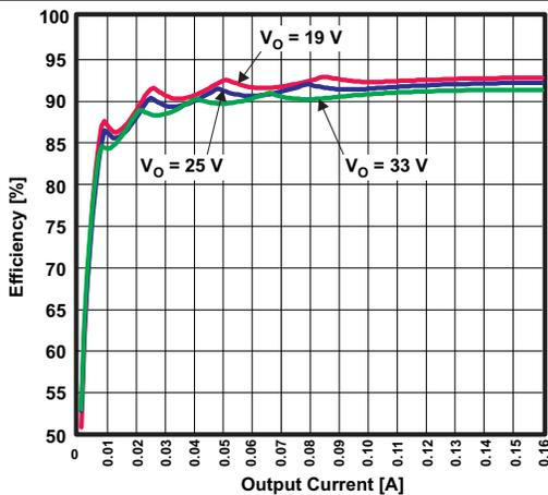
Figure 17. WLED Driver Efficiency vs Output Current
