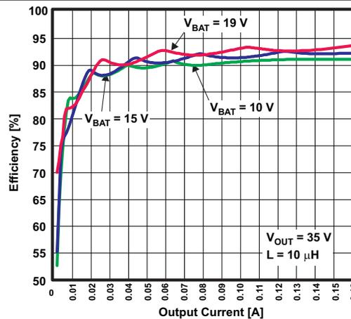
Figure 18. WLED Driver Efficiency vs Output Current
