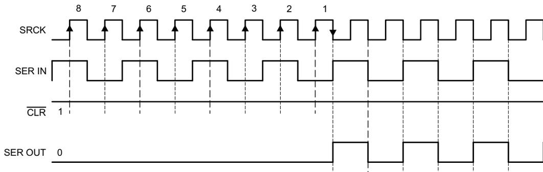
Figure 6-2. SER IN to SER OUT Waveform
