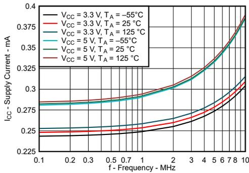
Figure 6-4. Supply Current vs Frequency
