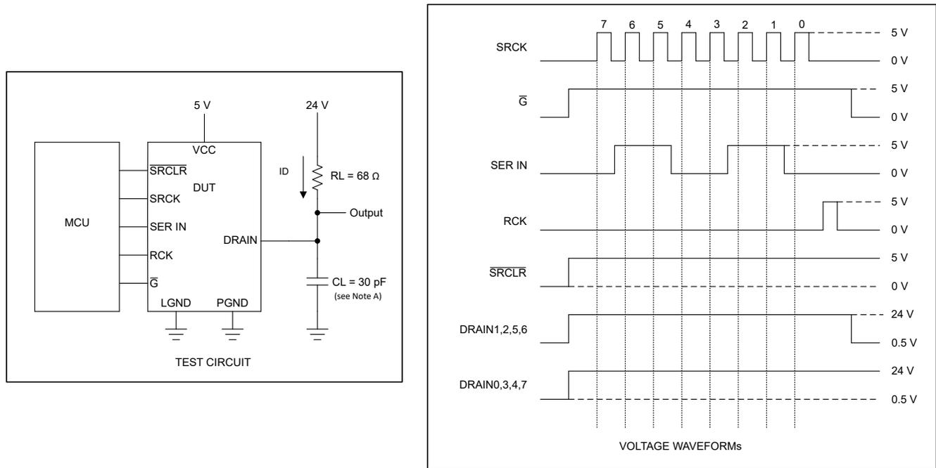
A.  $C_L$  includes probe and jig capacitance.
