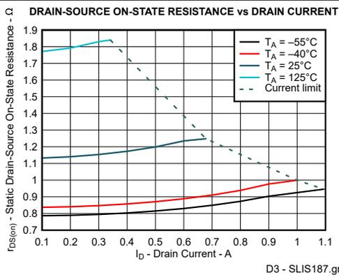
$V_{CC} = 3.3\text{ V}, T_A = 25\text{ }^\circ\text{C}$
