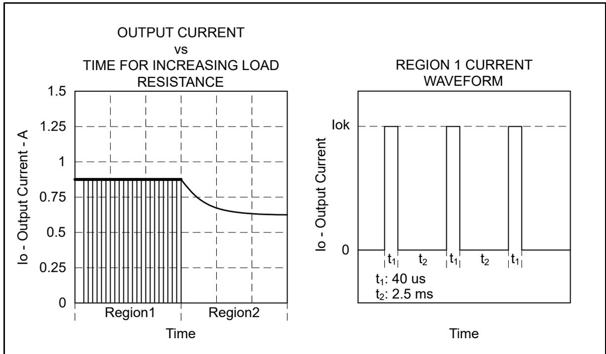
**Figure 8-2. Chopping-Mode Characteristics**
