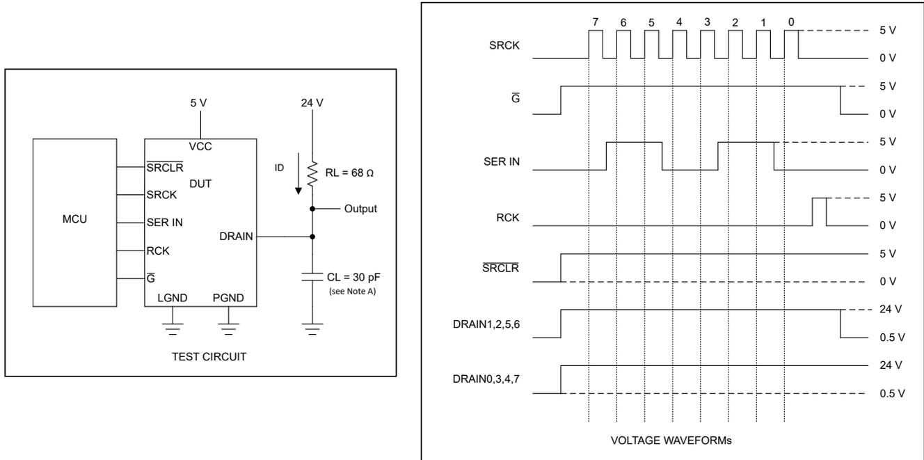
A.  $C_L$  includes probe and jig capacitance.
