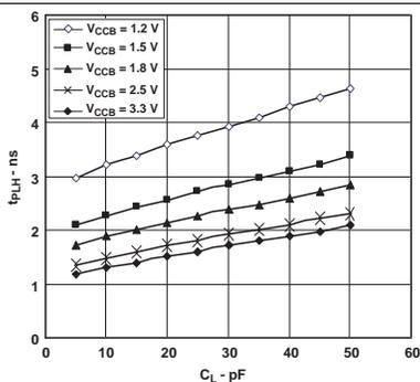
Figure 9. Typical A-to-B Propagation Delay, Low to High
