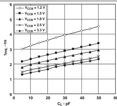
Figure 10. Typical A-to-B Propagation Delay, High to Low
