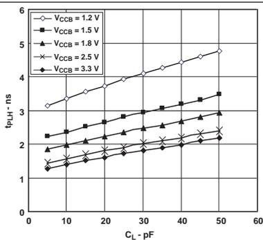
Figure 7. Typical A-to-B Propagation Delay, Low to High
