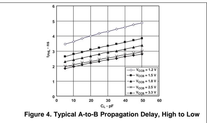
6.12.3 Typical Propagation Delay (A-to-B) vs Load Capacitance,  $T_A = 25^\circ\text{C}$ ,  $V_{CCA} = 1.8\text{ V}$
