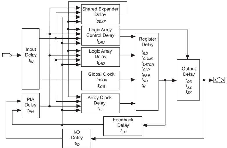
Timing information can be derived from the timing model and parameters for a particular EPLD. External timing parameters are calculated with the sum of internal parameters and represent pin-to-pin timing delays. Figure 8 shows the internal timing relationship for internal and external delay parameters.
