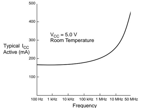
**Figure 9.  $I_{CC}$  vs. Frequency for MAX 5000 Devices (Part 2 of 2)**
