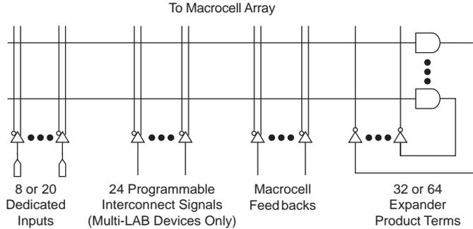
Expanders are fed by all signals in the LAB. One expander can feed all macrocells in the LAB or multiple product terms in the same macrocell. Because expanders also feed the secondary product terms of each macrocell, complex logic functions can be implemented without using additional macrocells. A small delay ( $t_{SEXP}$ ) is incurred when shared expanders are used.
