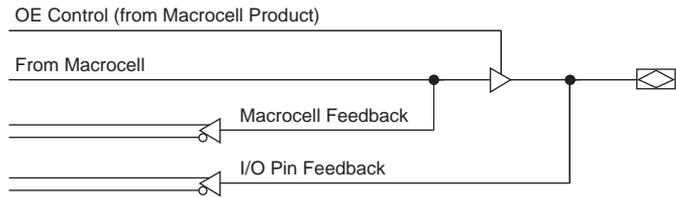
The MAX 5000 architecture provides dual I/O feedback in which macrocell and I/O pin feedbacks are independent, allowing maximum flexibility. When an I/O pin is configured as an input, the associated macrocell can be used for buried logic. Using an I/O pin as an input in single-LAB devices reduces the number of available expanders by two. In multi-LAB devices, I/O pins feed the PIA directly.
