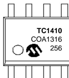
8-Lead MSOP (3x3 mm)
