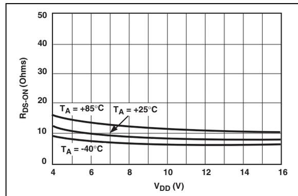
**FIGURE 2-6:** Low-State Output Resistance vs. Supply Voltage.
