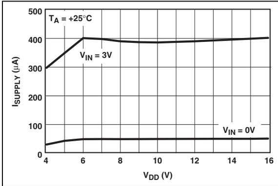
**FIGURE 2-1:** Quiescent Supply Current vs. Supply Voltage.
