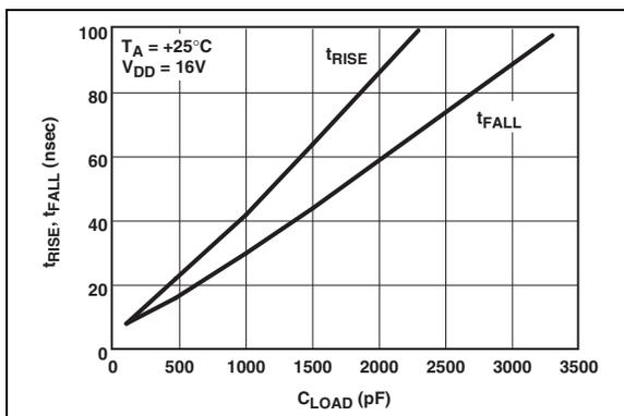
**FIGURE 2-9:** Rise and Fall Times vs. Capacitive Load.
