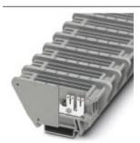
Feed-through terminal block, Connection method: Slip-on connection, Number of positions: 1, Cross section: 0.5 mm² - 6 mm², AWG: 20 - 10, Width: 23.2 mm, Color: gray, Mounting type: NS 35/7,5, NS 35/15
