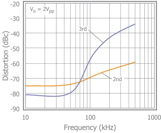
2nd & 3rd Harmonic Distortion at  $V_S = 2.7\text{V}$
