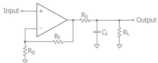
Figure 6. Addition of  $R_S$  for Driving Capacitive Loads
