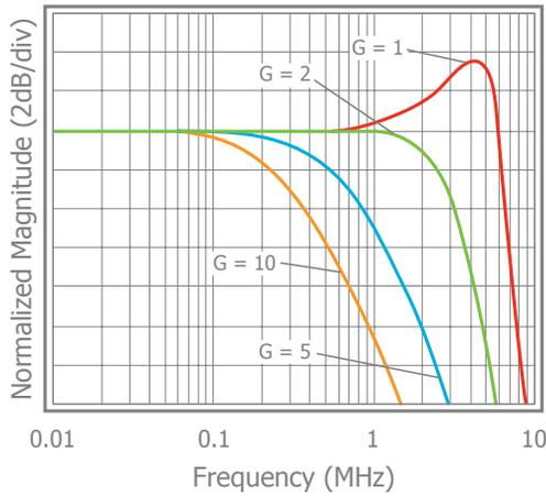
Inverting Frequency Response at  $V_S = 2.7\text{V}$
