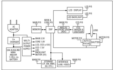
Figure 1. This compact digital-camera block diagram shows various operating voltages.
