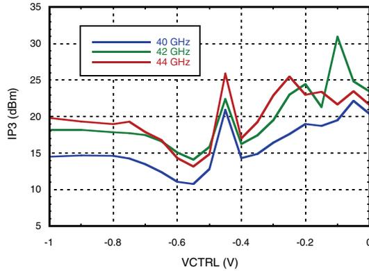
**Output IP3, LSB vs. Control Voltage [3]**
