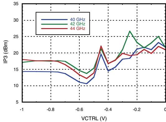
**Output IP3, LSB vs. Control Voltage [1]**
