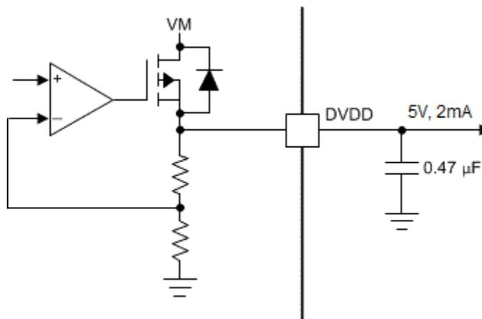
**Figure 7-10. Linear Voltage Regulator Block Diagram**
