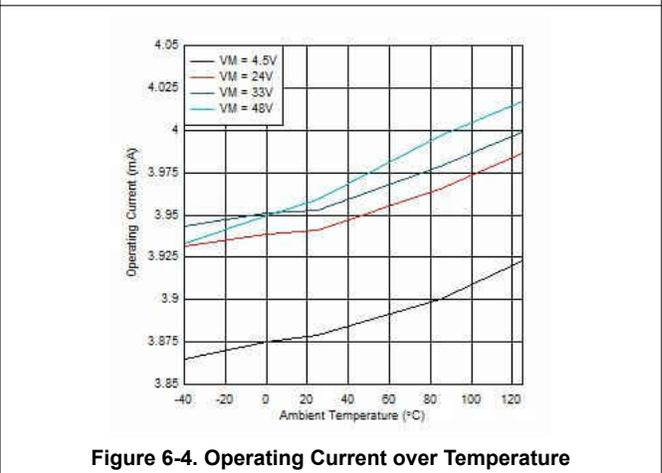
Figure 6-4. Operating Current over Temperature
