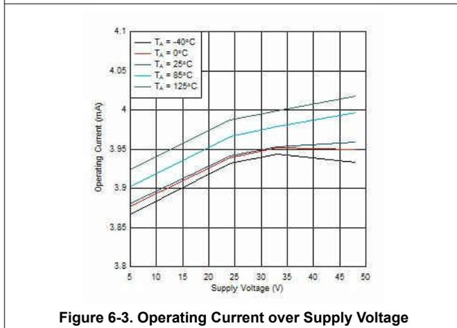
Figure 6-3. Operating Current over Supply Voltage
