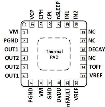
Figure 5-4. RGE Package 24-Pin VQFN with Exposed Thermal PAD Top View DRV8256P
