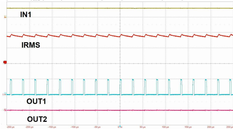
**Figure 8-4. Driver Full On Operation with Current Regulation**
