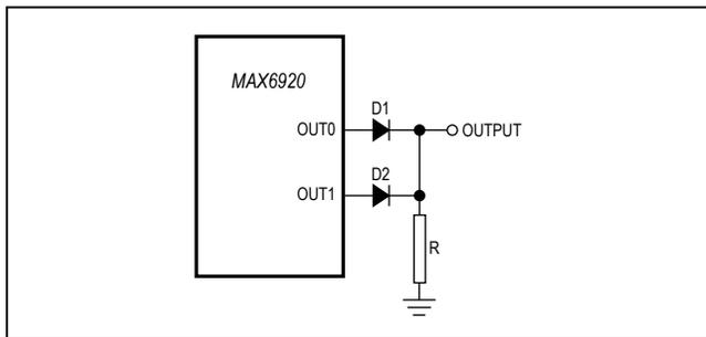
Figure 4. Paralleling Outputs
