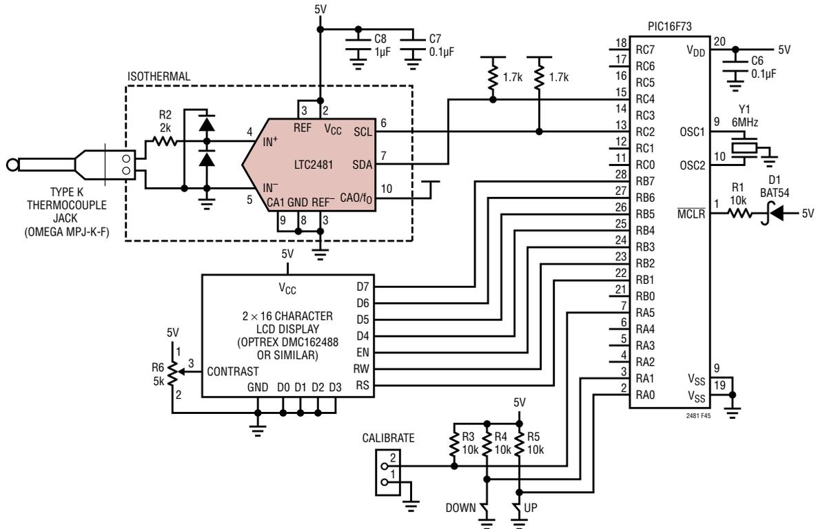
Figure 45. Complete Type K Thermocouple Meter
