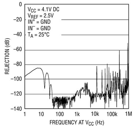
**PSRR vs Frequency at V<sub>CC</sub>**
