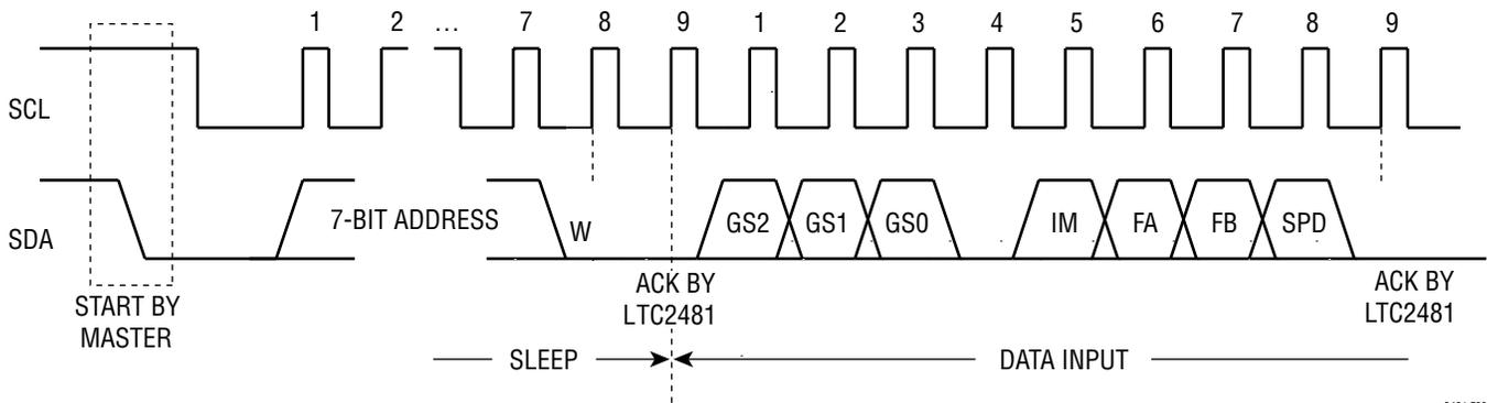
Figure 3. Timing Diagram for Writing to the LTC2481
