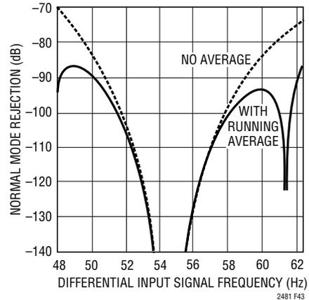
Figure 43. Input Normal Mode Rejection 2x Speed Mode
