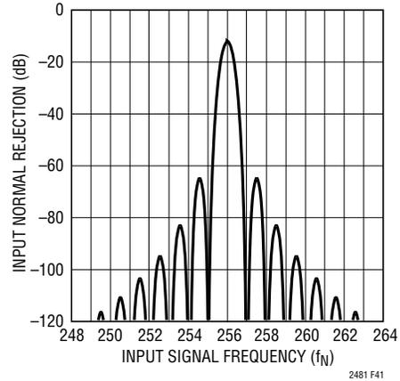
Figure 41. Input Normal Mode Rejection 2x Speed Mode
