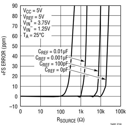
Figure 16. +FS Error vs R<sub>SOURCE</sub> at REF<sup>+</sup> or REF<sup>-</sup> (Small C<sub>REF</sub>)
