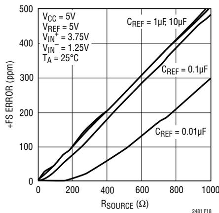
Figure 18. +FS Error vs R<sub>SOURCE</sub> at REF<sup>+</sup> or REF<sup>-</sup> (Large C<sub>REF</sub>)
