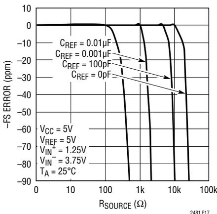
Figure 17. -FS Error vs R<sub>SOURCE</sub> at REF<sup>+</sup> or REF<sup>-</sup> (Small C<sub>REF</sub>)
