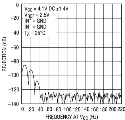
**PSRR vs Frequency at V<sub>CC</sub>**
