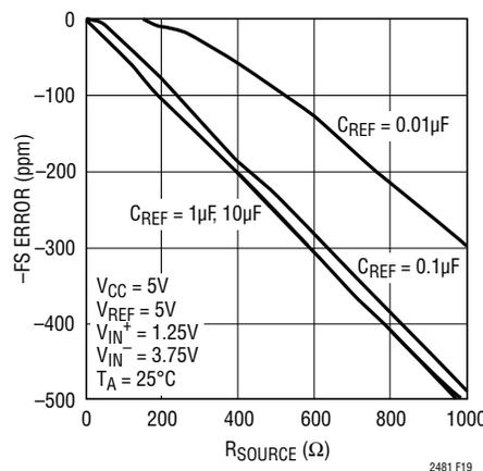
Figure 19. -FS Error vs R<sub>SOURCE</sub> at REF<sup>+</sup> or REF<sup>-</sup> (Large C<sub>REF</sub>)
