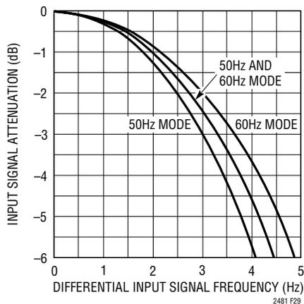
**Figure 29. Input Signal Using the Internal Oscillator**
