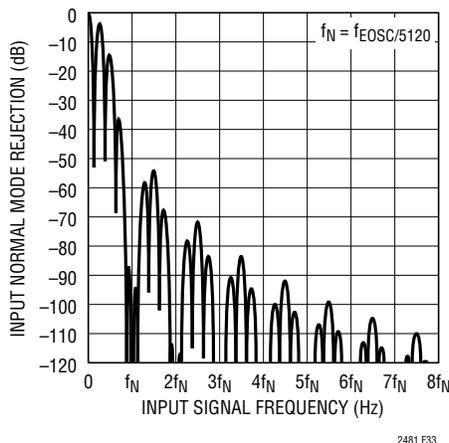
Figure 33. Input Normal Mode Rejection at DC
