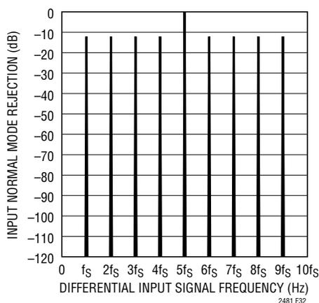
Figure 32. Input Normal Mode Rejection at DC
