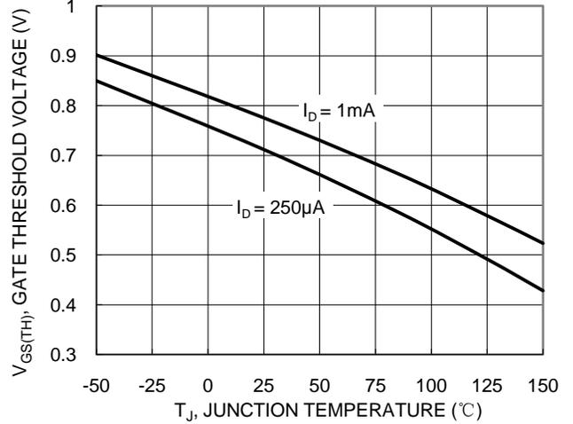
Figure 8. Gate Threshold Variation vs. Junction Temperature
