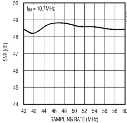
**ADC SIGNAL-TO-NOISE AND DISTORTION RATIO vs. SAMPLING RATE**
