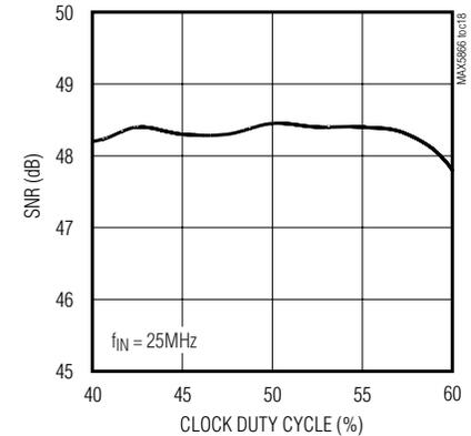
**ADC SIGNAL-TO-NOISE AND DISTORTION RATIO vs. CLOCK DUTY CYCLE**
