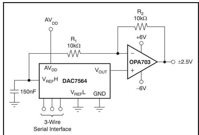
**Figure 100. Bipolar Output Range Using Internal Reference**
