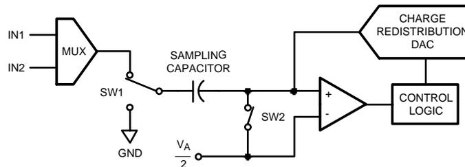
**Figure 46. ADC082S021 in Track Mode**
