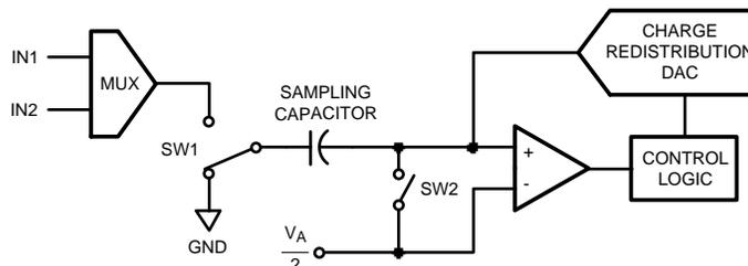
**Figure 47. ADC082S021 in Hold Mode**
