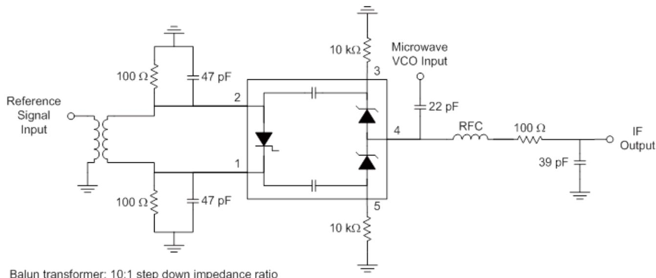
Balun transformer: 10:1 step down impedance ratio
