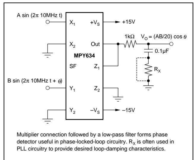
FIGURE 6. Phase Detector.
