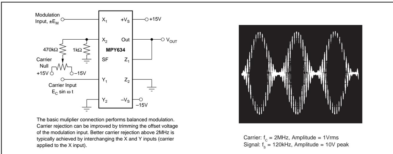
FIGURE 11. Balanced Modulator.
