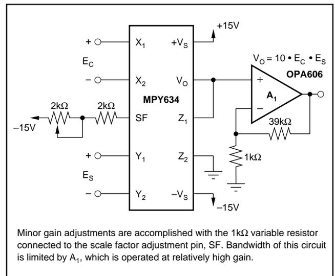
FIGURE 7. Voltage-Controlled Amplifier.
