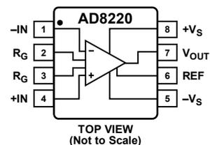
Figure 56. Pin Configuration
