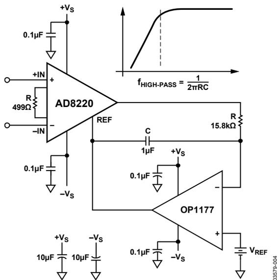
Figure 64. AC-Coupled Circuit
