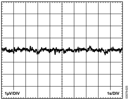
Figure 12. 0.1 Hz to 10 Hz RTI Voltage Noise (G = 1000)
