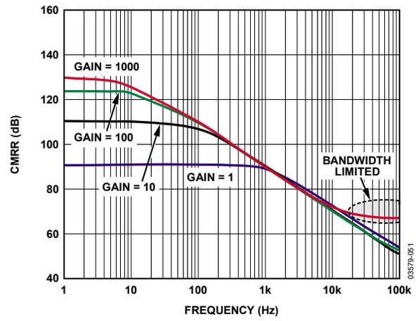
Figure 20. CMRR vs. Frequency, 1 kΩ Source Imbalance
