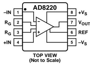
Figure 4. Pin Configuration
