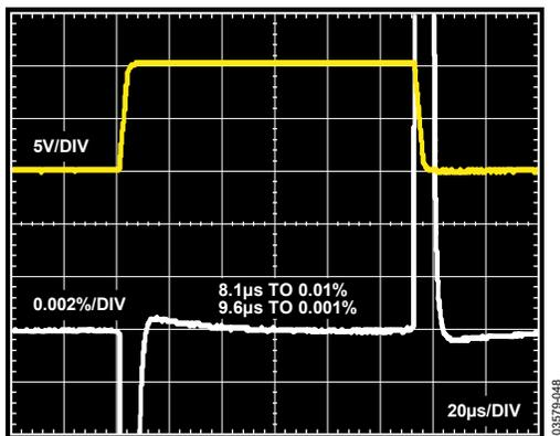
Figure 43. Large Signal Pulse Response and Settle Time,  $G = 100$ ,  $R_{LOAD} = 10\text{ k}\Omega$ ,  $V_S = \pm 15\text{ V}$ ,  $V_{REF} = 0\text{ V}$
