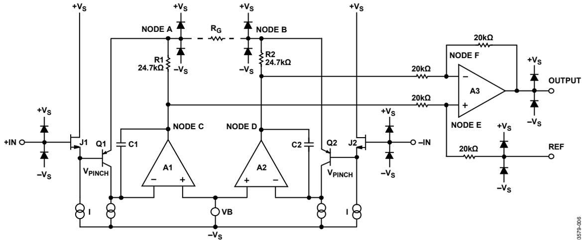
Figure 55. Simplified Schematic
