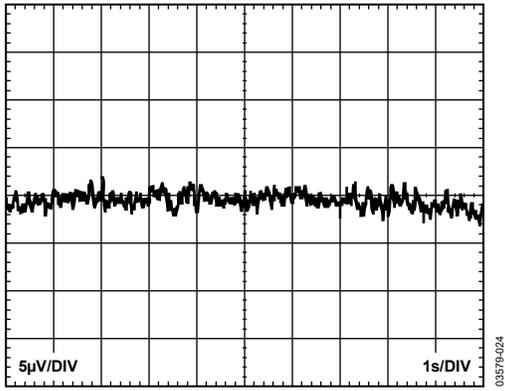
Figure 11. 0.1 Hz to 10 Hz RTI Voltage Noise (G = 1)
