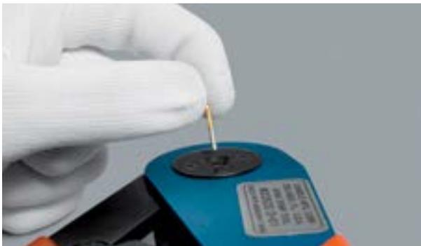
Insert the contact into the crimping tool.
