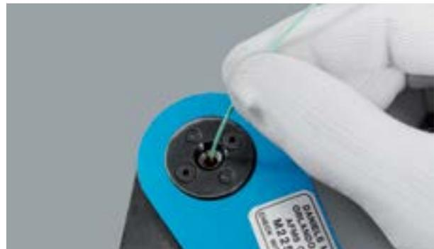
Insert the wire into the contact.
