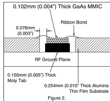
**General Handling:** Handle the chip along the edges with a vacuum collet or with a sharp pair of bent tweezers. The surface of the chip may have fragile air bridges and should not be touched with vacuum collet, tweezers, or fingers.
