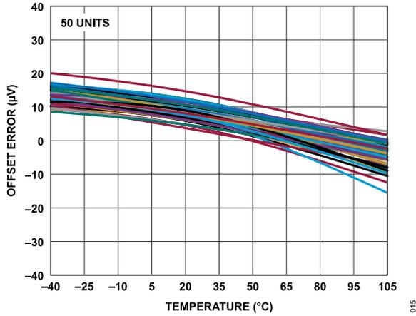
Figure 15. Offset Error vs. Temperature (Gain = 1, Before Calibration)
