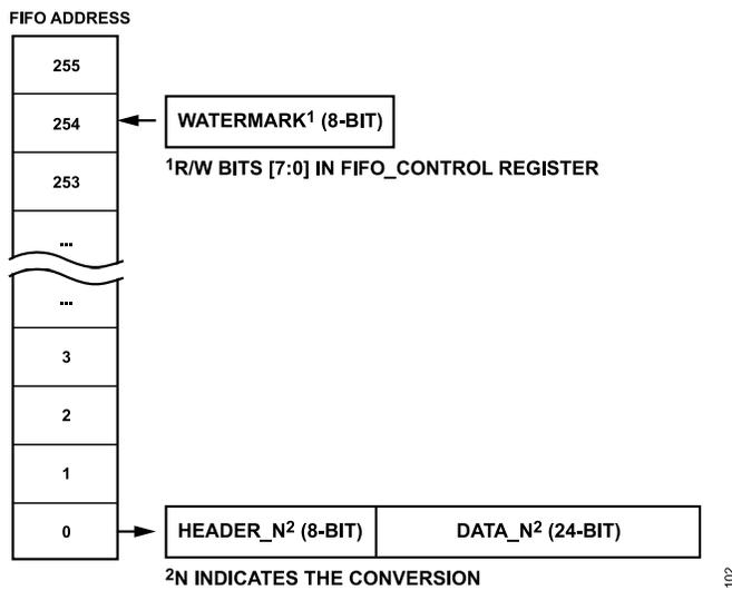
Figure 102. FIFO Structure
