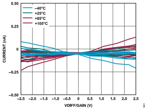
Figure 41. Differential AIN Current vs. VDIFF/Gain for Various Temperatures (Gain = 2 to 128, VCM = AV<sub>DD</sub>/2)
