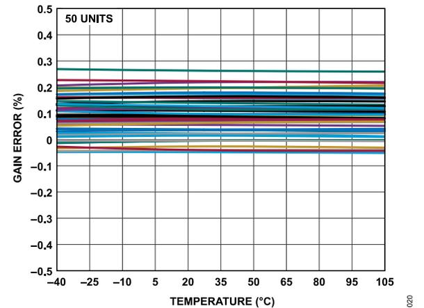
Figure 20. Gain Error vs. Temperature (Gain = 32, Before Calibration)
