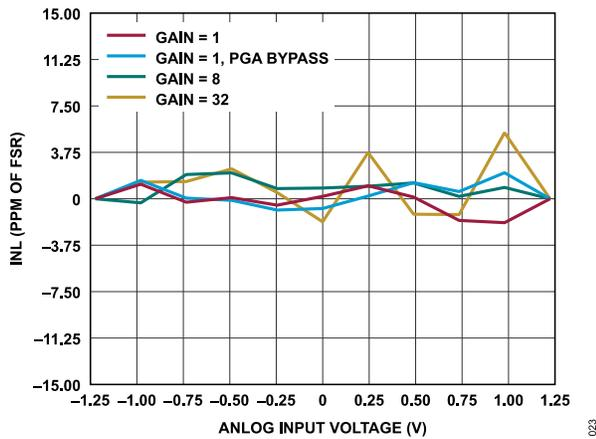
Figure 23. INL Error vs. Differential Input Amplitude for Various Gains (Sinc<sup>3</sup> Filter, ODR = 50 SPS, AV<sub>DD</sub> = 1.8 V, Internal 1.25 V Reference)
