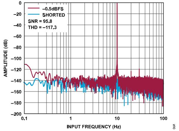
Figure 68. FFT, -0.5 dBFS vs. Shorted Inputs, 10 Hz Input Tone, Sinc<sup>3</sup> Filter, ODR = 240 SPS, Gain = 1, External Reference
