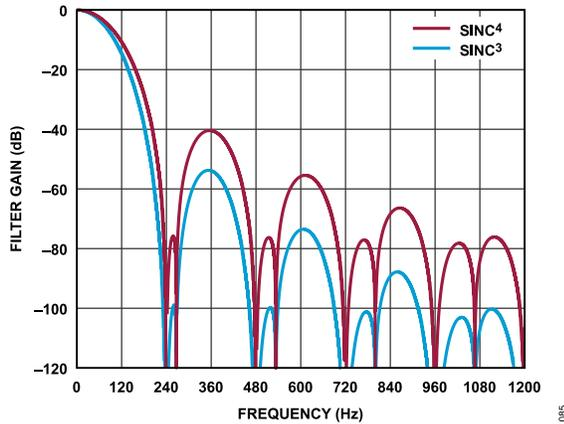
Figure 85. Sinc<sup>3</sup> and Sinc<sup>4</sup> Filter Response (FS = 0d10)
