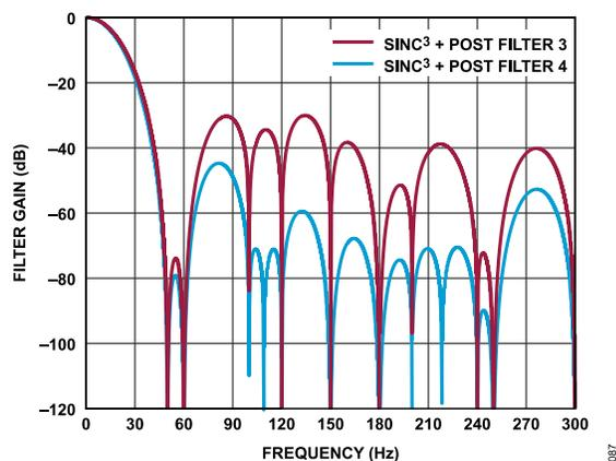
Figure 87. Post Filter 3 and Post Filter 4 Response
