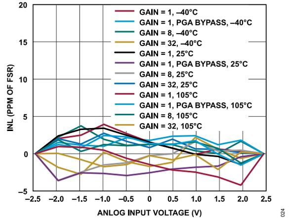
Figure 24. INL Error vs. Differential Input Amplitude for Various Gains and Temperatures (Sinc<sup>3</sup> Filter, ODR = 50 SPS, Internal 2.5 V Reference)
