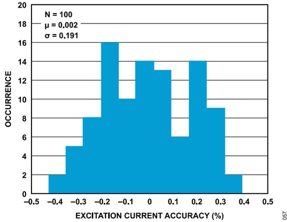
Figure 57. Excitation Current Initial Accuracy Histogram (100 μA)
