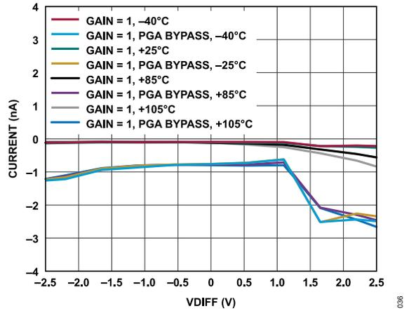
Figure 36. Absolute AINM Current vs. VDIFF for Various Temperatures (Gain = 1, VCM = AV<sub>DD</sub>/2)
