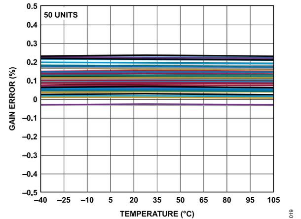
Figure 19. Gain Error vs. Temperature (Gain = 8, Before Calibration)
