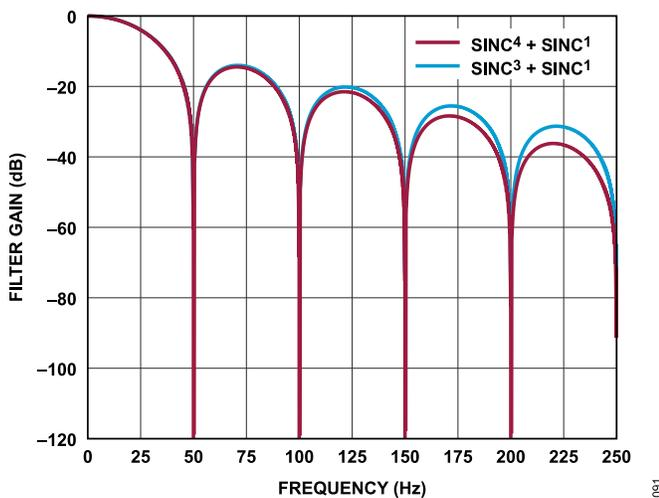
Figure 91. Sinc<sup>3</sup> + Sinc<sup>1</sup> and Sinc<sup>4</sup> + Sinc<sup>1</sup> Filter Response (FS = 6)
