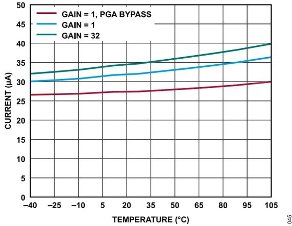
Figure 45.  $AV_{DD}$  Current vs. Temperature for Various Gains
