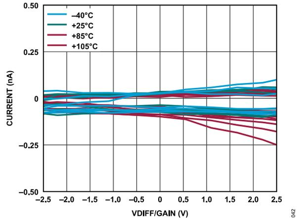
Figure 42. Absolute AINM Current vs. VDIFF/Gain for Various Temperatures (Gain = 2 to 128, VCM = AV<sub>DD</sub>/2)
