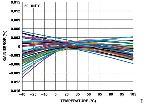
Figure 18. Gain Error vs. Temperature (Gain = 1, Factory Calibrated)
