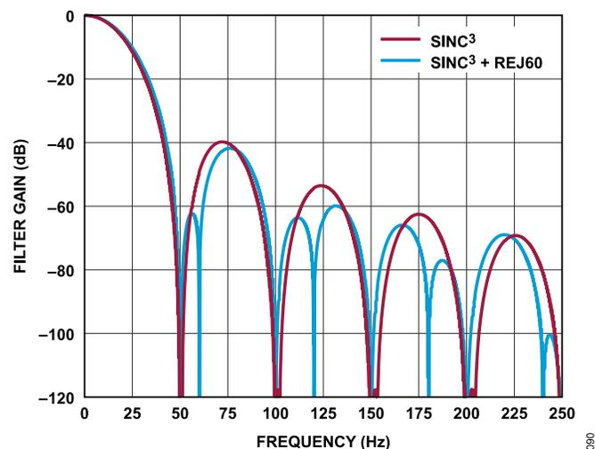
Figure 90. Sinc<sup>3</sup> and Sinc<sup>3</sup> + REJ60 Filter Response (50 SPS ODR)
