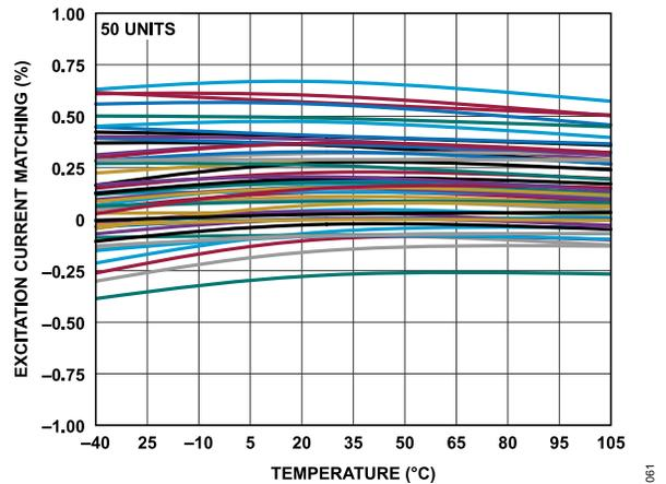
Figure 61. Excitation Current Matching vs. Temperature (100 μA)
