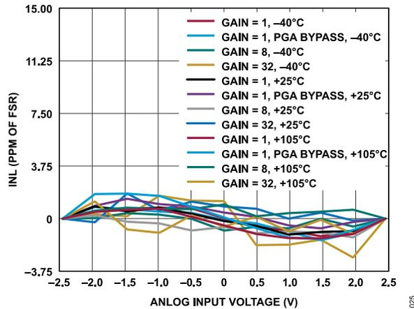
Figure 25. INL Error vs. Differential Input Amplitude for Various Gains and Temperatures (Sinc<sup>3</sup> Filter, ODR = 50 SPS, External 2.5 V Reference)
