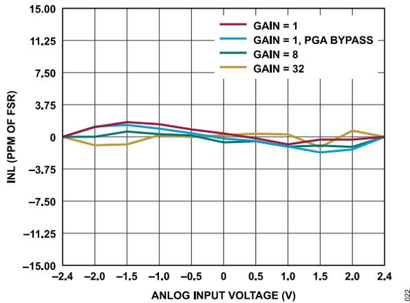
Figure 22. INL Error vs. Differential Input Amplitude for Various Gains (Sinc<sup>3</sup> Filter, ODR = 50 SPS, External 2.5 V Reference)
