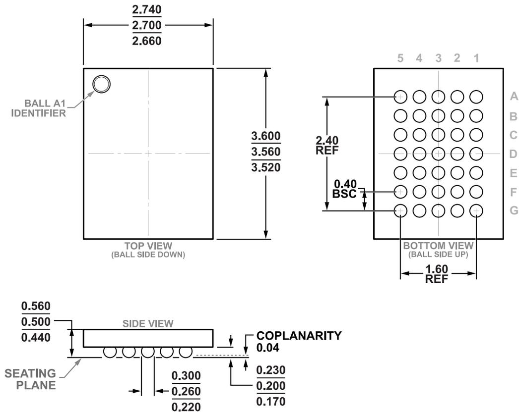
Figure 127. 35-Ball Wafer Level Chip Scale Package [WLCSP]
