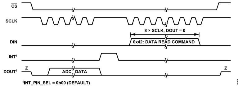
Figure 82. Exit Continuous Read Mode Diagram (CRC Disabled)
