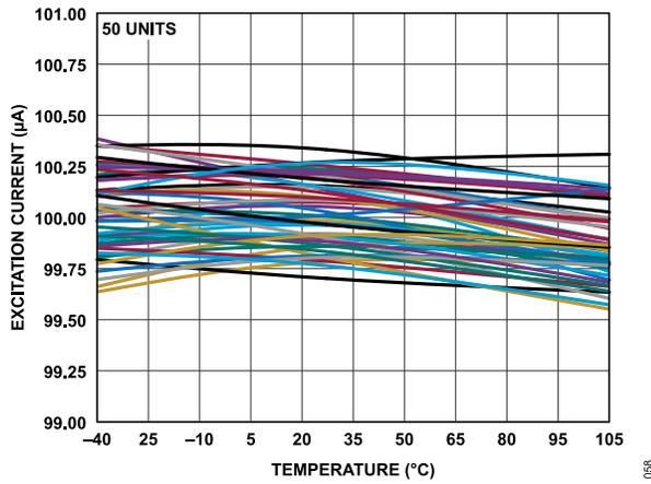
Figure 58. Excitation Current vs. Temperature (100 μA)
