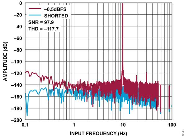
Figure 67. FFT, -0.5 dBFS vs. Shorted Inputs, 10 Hz Input Tone, Sinc<sup>3</sup> Filter, ODR = 240 SPS, Gain = 1, Internal Reference
