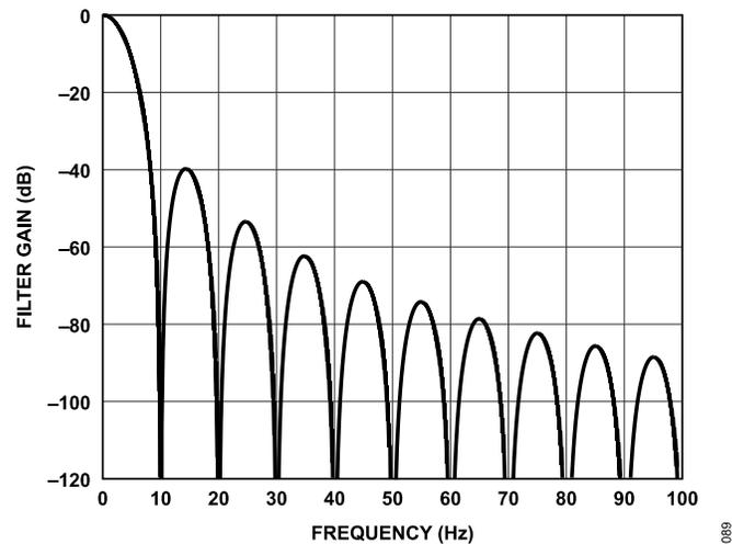
Figure 89. Simultaneous 50 Hz and 60 Hz Rejection for Sinc<sup>3</sup> with ODR = 10 SPS
