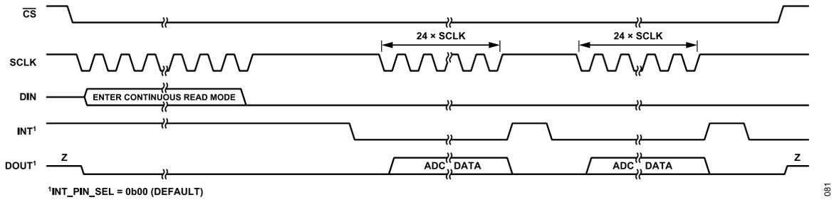
Figure 81. Enter Continuous Read Mode Diagram (DATA\_STATUS = 0)
