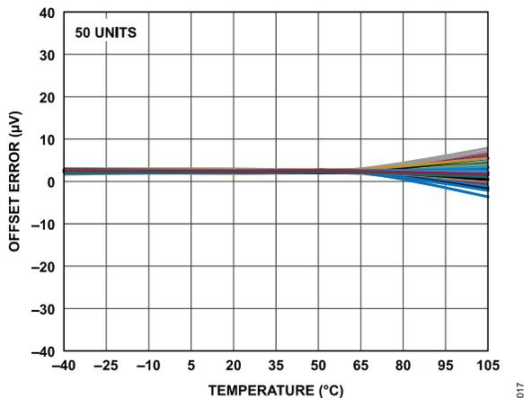
Figure 17. Offset Error vs. Temperature (Gain = 32, Before Calibration)
