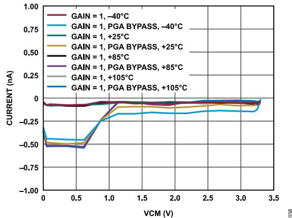
Figure 38. Differential AIN Current vs. VCM for Various Temperatures (Gain = 1, VCM = AV<sub>DD</sub>/2)
