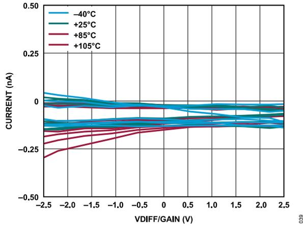
Figure 39. Absolute AINP Current vs. Normalized Differential AIN Voltage (VDIFF/Gain) for Various Temperatures (Gain = 2 to 128, VCM = AV<sub>DD</sub>/2)
