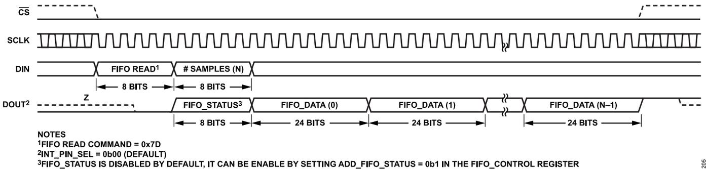
Figure 105. FIFO Readback (FIFO\_STATUS Append On and FIFO\_HEADER Append Off)
