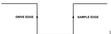
Figure 72. SPI Mode 3, SCLK Edges
