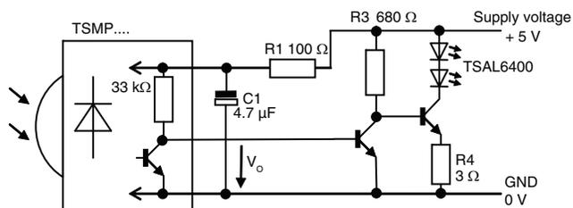
Recommended circuit for best sensitivity of the TSMP.... in repeater applications. It limits the output voltage swing V<sub>o</sub> to about 0.7 V in order to avoid internal coupling.
