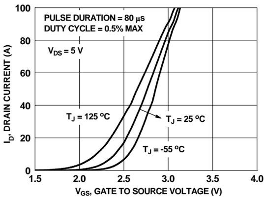
Figure 18. Transfer Characteristics
