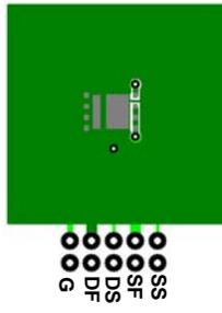
b. 50 °C/W when mounted on a 1 in<sup>2</sup> pad of 2 oz copper
