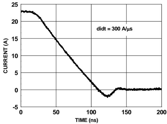
Figure 27. FDMS3686S SyncFET body diode reverse recovery characteristic
