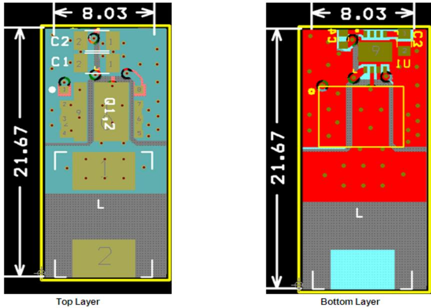
Figure 31. Recommended PCB Layout
