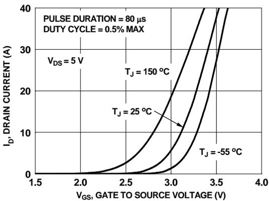
Figure 5. Transfer Characteristics
