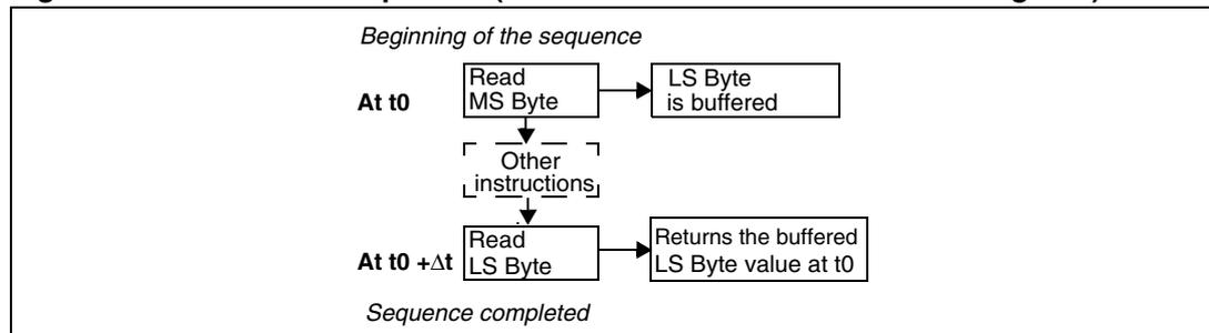
The user must read the MS Byte first, then the LS Byte value is buffered automatically.
