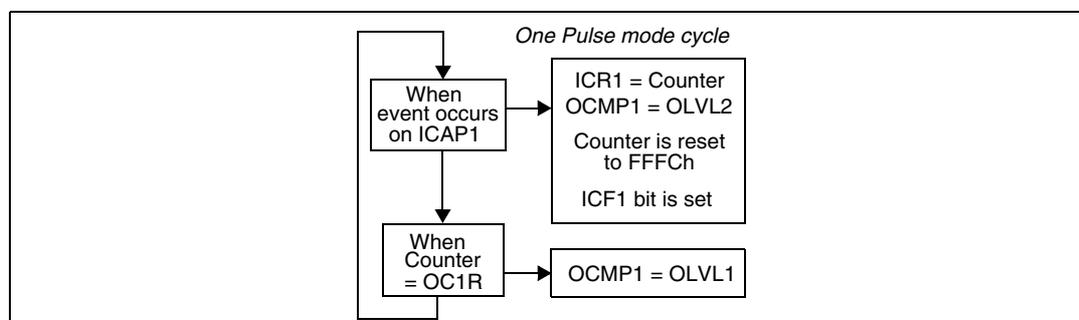
Then, on a valid event on the ICAP1 pin, the counter is initialized to FFFCh and OLVL2 bit is loaded on the OCMP1 pin, the ICF1 bit is set and the value FFFDh is loaded in the IC1R register.
