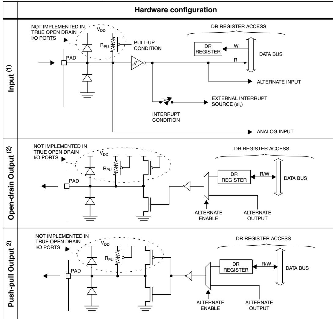
1. When the I/O port is in input configuration and the associated alternate function is enabled as an output, reading the DR register will read the alternate function output status.
