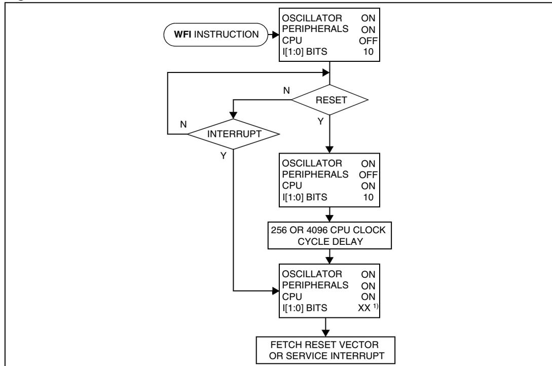
Note: Before servicing an interrupt, the CC register is pushed on the stack. The I[1:0] bits of the CC register are set to the current software priority level of the interrupt routine and recovered when the CC register is popped.
