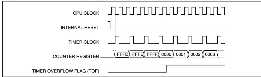
**Figure 50. Counter timing diagram, internal clock divided by 4**
