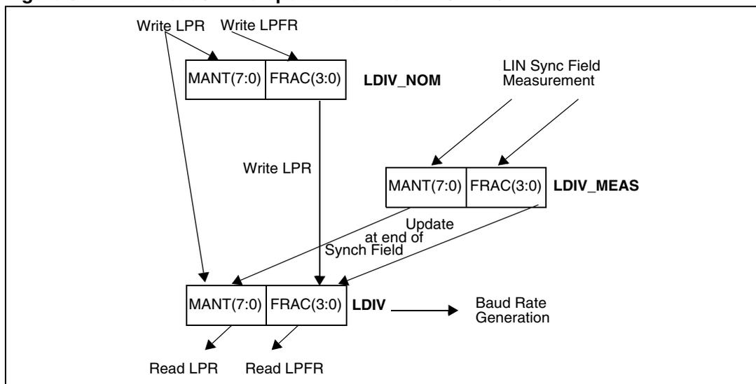
Figure 85. LDIV read / write operations when LDUM = 1
