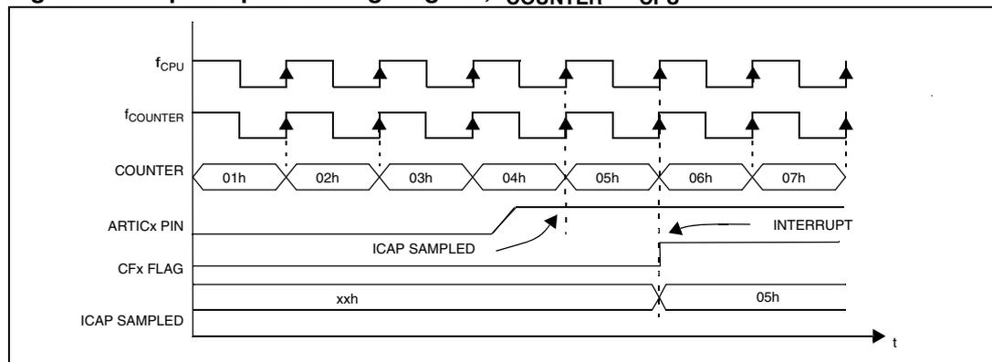
Figure 45. Input capture timing diagram,  $f_{\text{COUNTER}} = f_{\text{CPU}} / 4$
