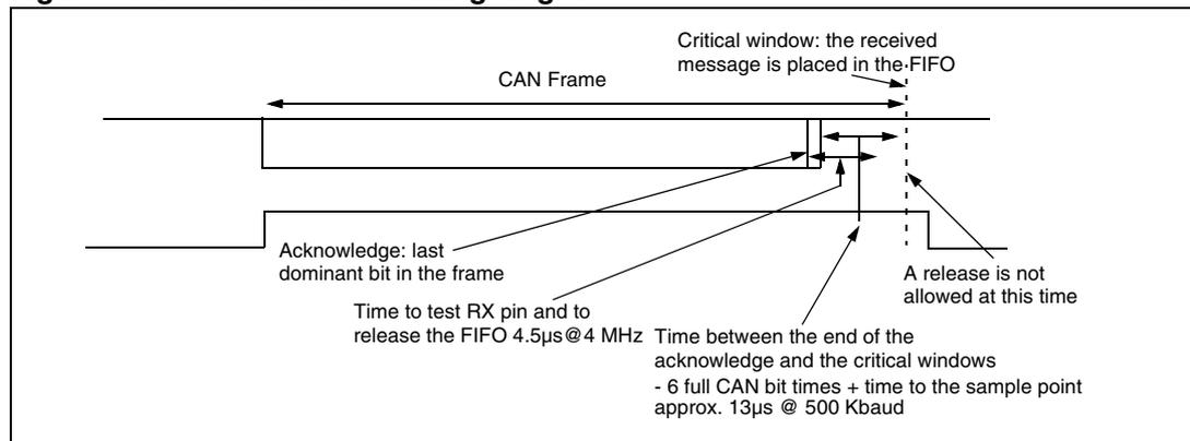
**Figure 112. Reception of a sequence of frames**
