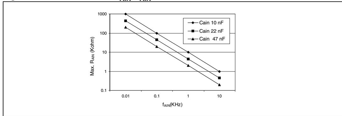
1. Figure 143 shows that depending on the input signal variation ( $f_{AIN}$ ),  $C_{AIN}$  can be increased for stabilization time and reduced to allow the use of a larger serial resistor ( $R_{AIN}$ ). It is valid for all  $f_{ADC}$  frequencies  $\leq 4$  MHz.
