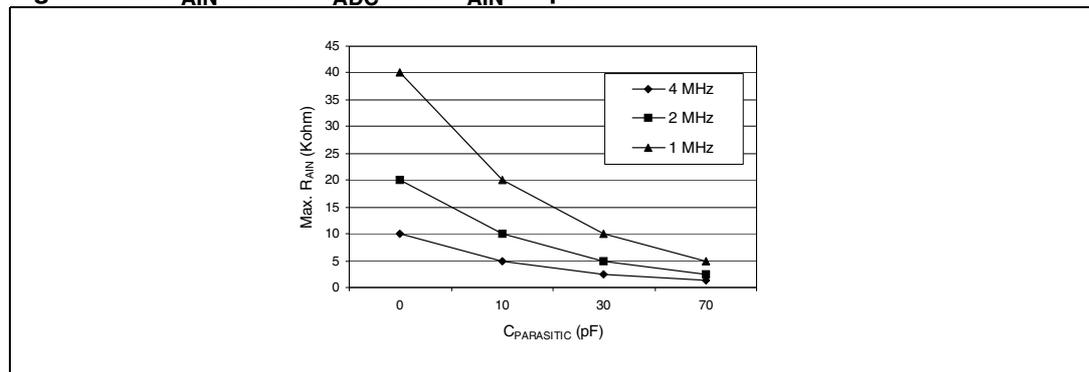
1. C<sub>PARASITIC</sub> represents the capacitance of the PCB (dependent on soldering and PCB layout quality) plus the pad capacitance (3pF). A high C<sub>PARASITIC</sub> value will downgrade conversion accuracy. To remedy this, f<sub>ADC</sub> should be reduced.
