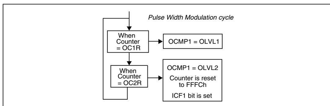
If OLVL1 = 1 and OLVL2 = 0 the length of the positive pulse is the difference between the OC2R and OC1R registers.
