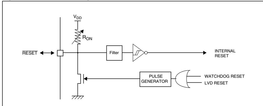
The  $\overline{\text{RESET}}$  pin is an asynchronous signal which plays a major role in EMS performance. In a noisy environment, it is recommended to follow the guidelines mentioned in the electrical characteristics section.
