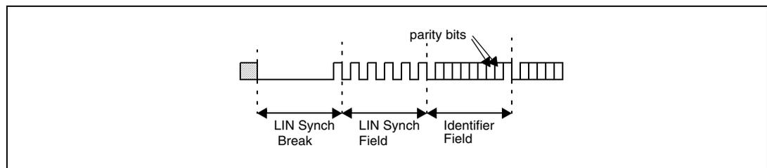
The bits involved are the two MSB positions (7th and 8th bits if M = 0; 8th and 9th bits if M = 0) of the identifier character. The check is performed as specified by the LIN specification:
