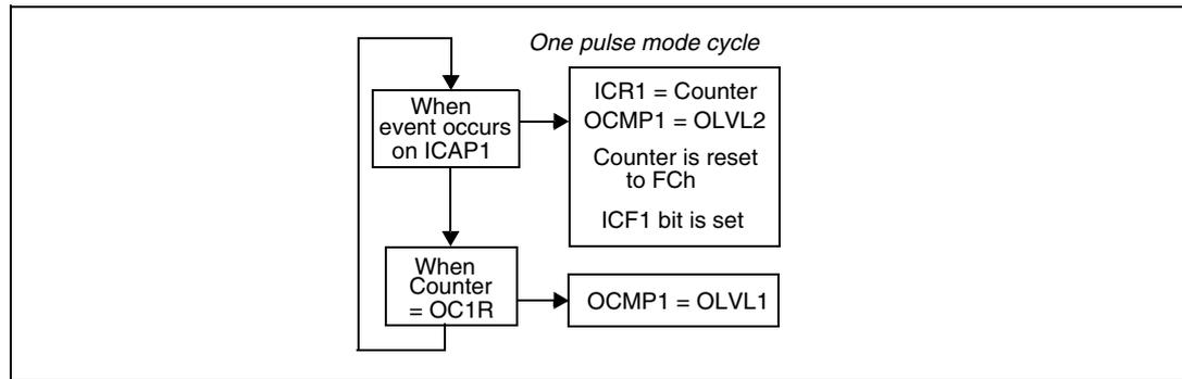
Then, on a valid event on the ICAP1 pin, the counter is initialized to FCh and OLVL2 bit is loaded on the OCMP1 pin, the ICF1 bit is set and the value FFFDh is loaded in the IC1R register.
