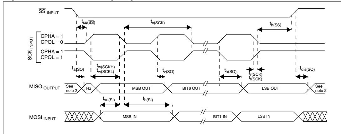
1. Measurement points are done at CMOS levels:  $0.3 \times V_{DD}$  and  $0.7 \times V_{DD}$ .
