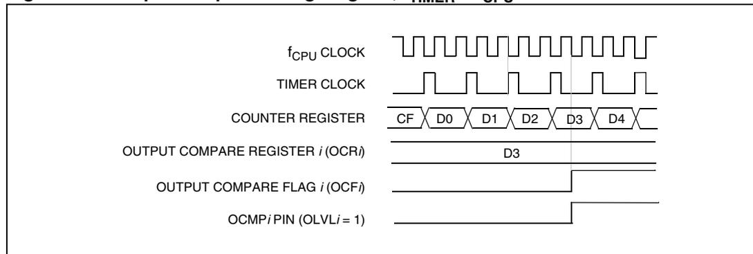
Figure 67. Output compare timing diagram,  $f_{\text{TIMER}} = f_{\text{CPU}}/4$
