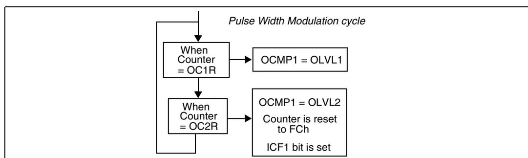
If OLVL1 = 1 and OLVL2 = 0 the length of the positive pulse is the difference between the OC2R and OC1R registers.
