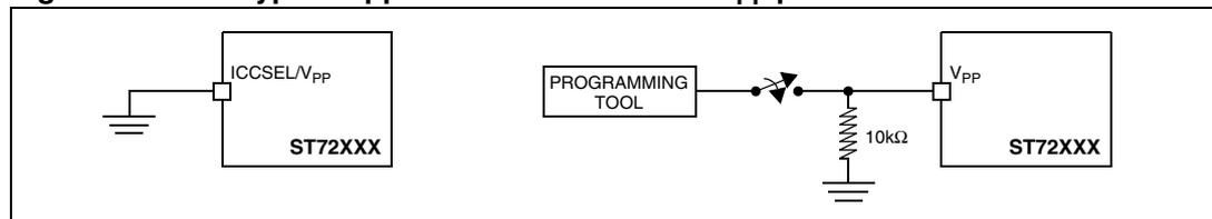
1. When ICC mode is not required by the application ICCSEL/V<sub>PP</sub> pin must be tied to V<sub>SS</sub>.
