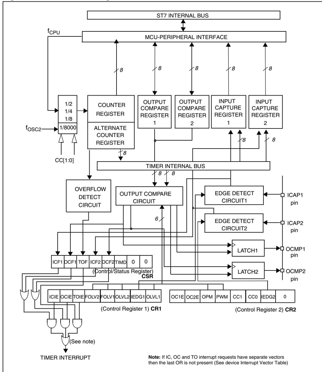
Whatever the timer mode used (input capture, output compare, one pulse mode or PWM mode) an overflow occurs when the counter rolls over from FFh to 00h then:
