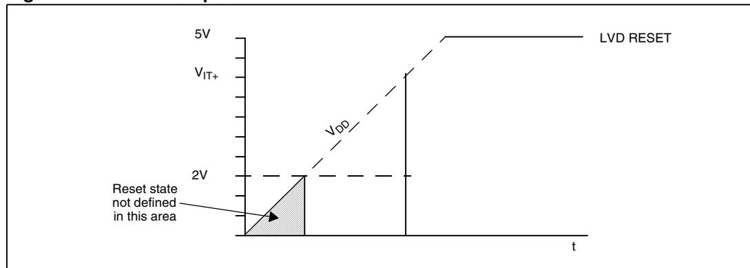
*Note:* When the LVD is enabled, the MCU reaches its authorized operating voltage from a reset state. However, in some devices, the reset signal may be undefined until  $V_{DD}$  is approximately 2V. As a consequence, the I/Os may toggle when  $V_{DD}$  is below this voltage.
