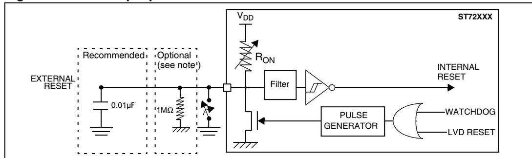
**Note:** When the LVD is enabled, it is mandatory not to connect a pull-up resistor. A 10nF pull-down capacitor is recommended to filter noise on the reset line. In case a capacitive power supply is used, it is recommended to connect a 1 MΩ pull-down resistor to the RESET pin to discharge any residual voltage induced by this capacitive power supply (this will add 5 μA to the power consumption of the MCU).
