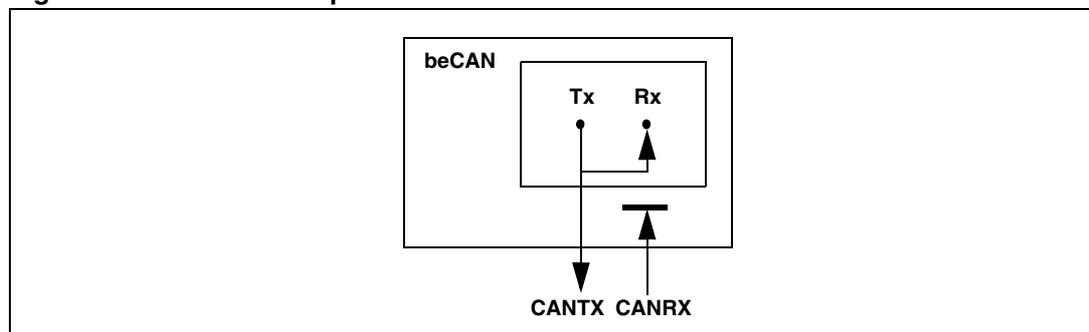
This mode is provided for self-test functions. To be independent of external events, the CAN core ignores acknowledge errors (no dominant bit sampled in the acknowledge slot of a data
