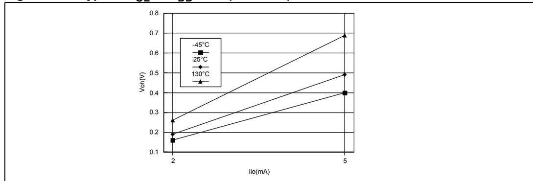
**Figure 130. Typical  $V_{OL}$  at  $V_{DD} = 5V$  (high-sink)**
