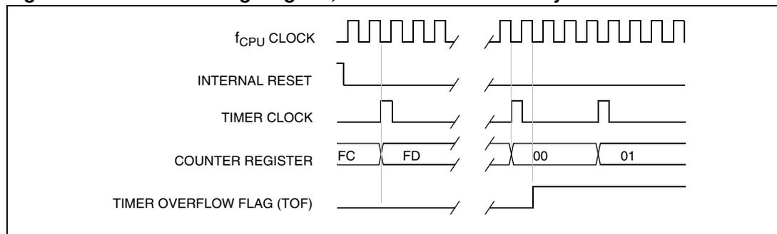
**Figure 62. Counter timing diagram, internal clock divided by 8**
