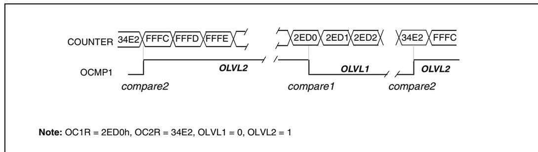
Note: On timers with only one Output Compare register, a fixed frequency PWM signal can be generated using the output compare and the counter overflow to define the pulse length.
