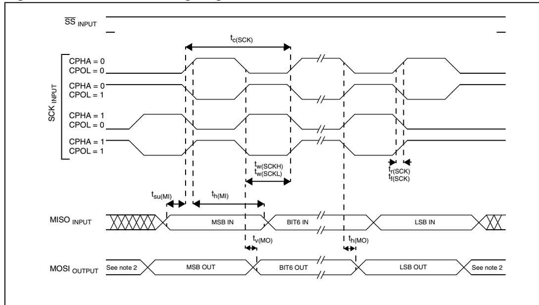
1. Measurement points are done at CMOS levels:  $0.3 \times V_{DD}$  and  $0.7 \times V_{DD}$ .
