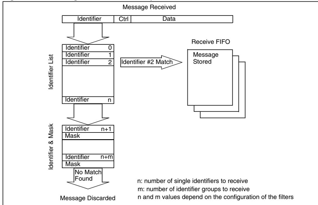
The example above shows the filtering principle of the beCAN. On reception of a message, the identifier is compared first with the filters configured in identifier list mode. If there is a match, the message is stored in the FIFO and the index of the matching filter is stored in the filter match index. As shown in the example, the identifier matches with identifier #2 thus the message content and MFMI 2 is stored in the FIFO.
