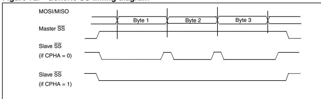
**Figure 73. Hardware/software slave select management**
