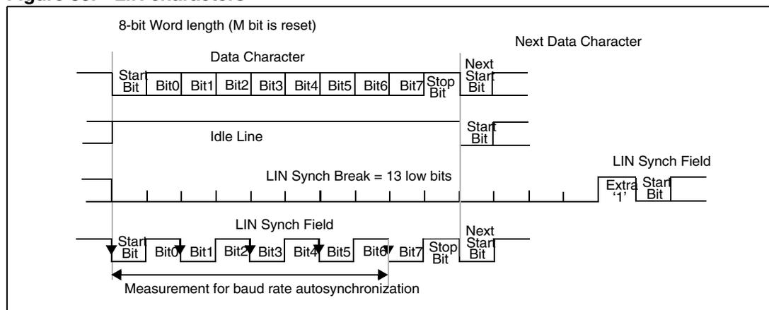
Figure 81. SCI block diagram in LIN slave mode
