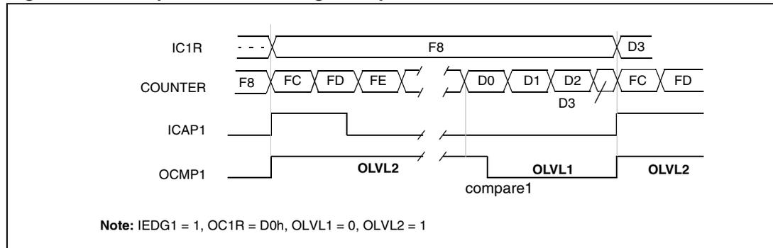
**Figure 69. Pulse width modulation mode timing example**
