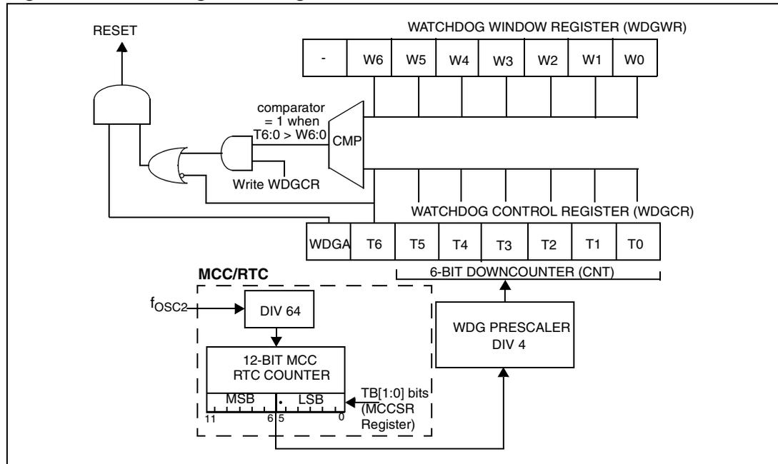
The application program must write in the WDGCR register at regular intervals during normal operation to prevent an MCU reset. This operation must occur only when the counter value is lower than the window register value. The value to be stored in the WDGCR register must be between FFh and C0h (see [Figure 35](#)):
