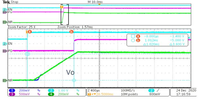
$V_{in}=6.5\text{V}$ ,  $I_o=1\text{A}$ , EN to PG=1ms.  $C_{NRSS}=1\text{nF}$ .
