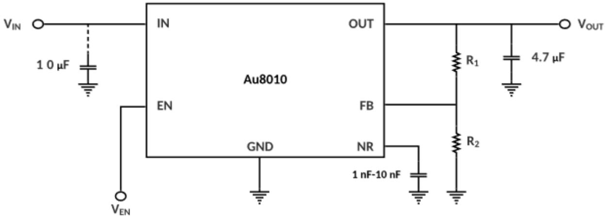
Figure 4 Typical Application Adjustable Voltage
