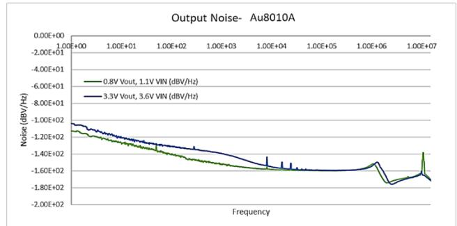
Conditions:  $C_{out}=10\text{ }\mu\text{F}$ ,  $C_{nrss}=100\text{ nF}$ ,  $C_{ff}=10\text{ nF}$ ,  $I_{out}=1\text{ A}$ ,  $V_{IN}=V_{out}+0.3\text{V}$
