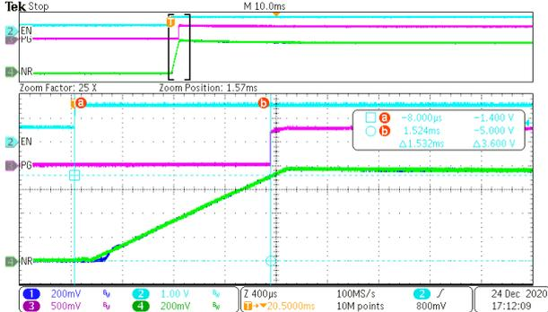
$V_{in}=6.5\text{V}$ ,  $I_o=5\text{mA}$ , EN to PG=1.53ms.  $C_{NRSS}=1\text{nF}$ .
