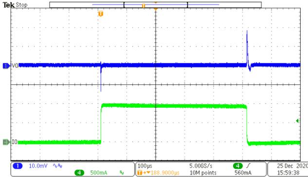
$V_{in}=1.1\text{V}$ ,  $V_o=0.8\text{V}$ ,  $C_{NR}=1\text{nF}$ ,  $C_{ff}=0$ ,  $C_{out}=10\text{ }\mu\text{F}$  (5mA  $\rightarrow$  1A  $\rightarrow$  5mA). Slew rate: 1A/ $\mu\text{s}$ .
