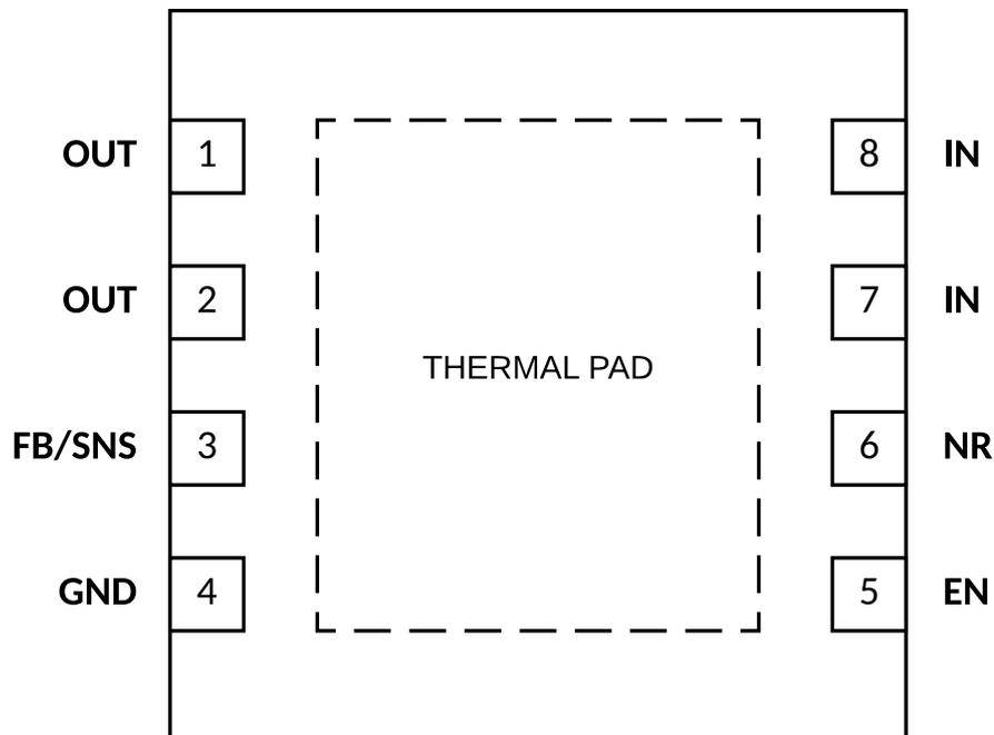
Figure 2 Au8010A Pin Configuration
