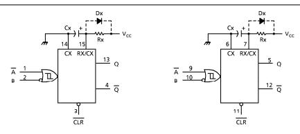
Notes: (1) Cx, Rx, Dx are external Capacitor, Resistor, and Diode, respectively.
