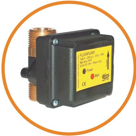
The FSP10 is designed for directly controlling an electric pump that is providing increased pressure or flow within water systems that are gravity fed from storage tanks. The device has to be fitted in the pipe above the pump.
