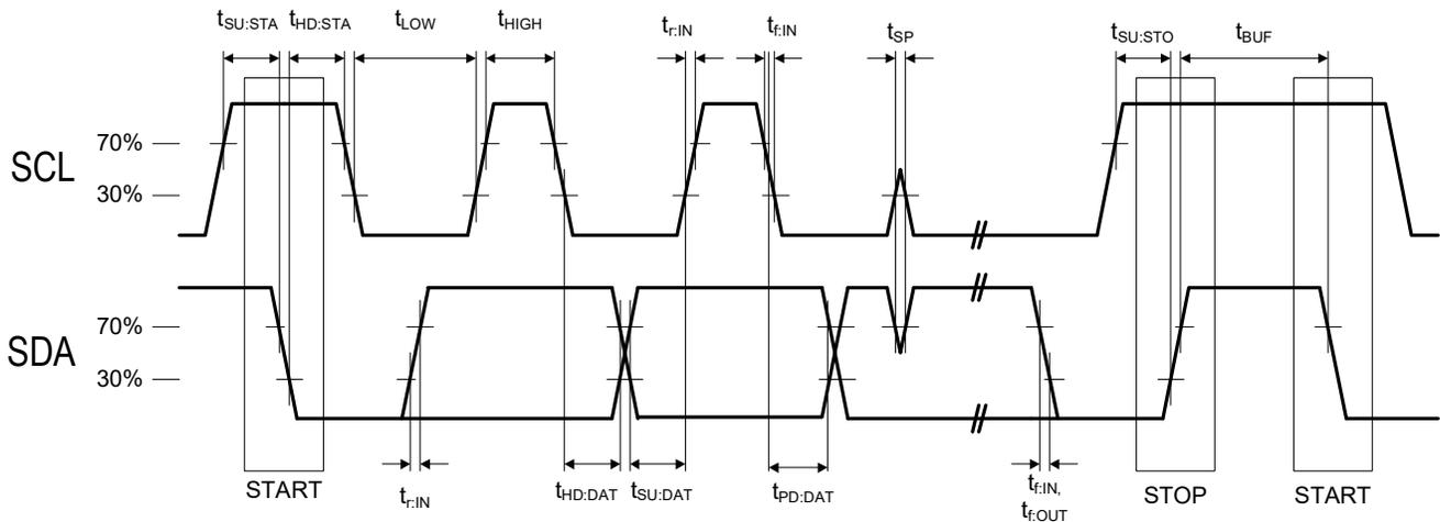
**Figure 3. I<sup>2</sup>C Control Interface Read and Write Timing Parameters**
