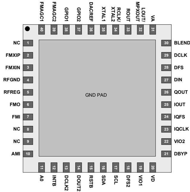
**Figure 23. Si4777 Pin Descriptions for IBOC Blend Mode**
