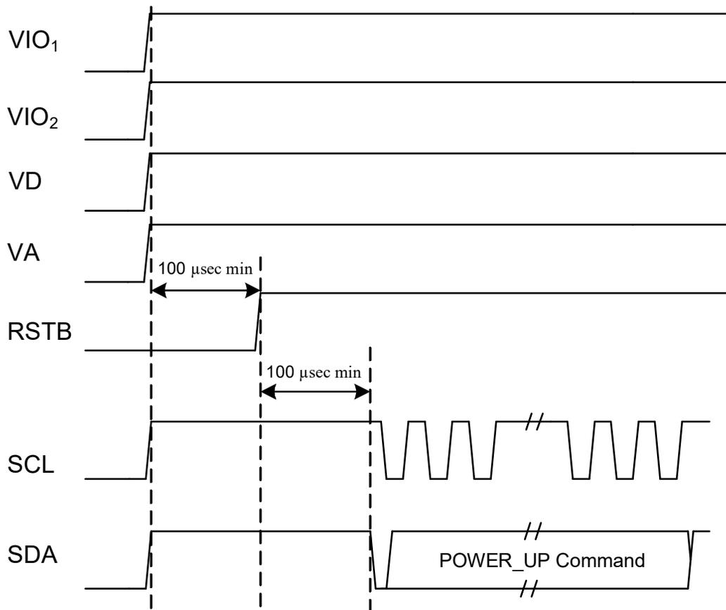
Figure 27. Startup Timing
