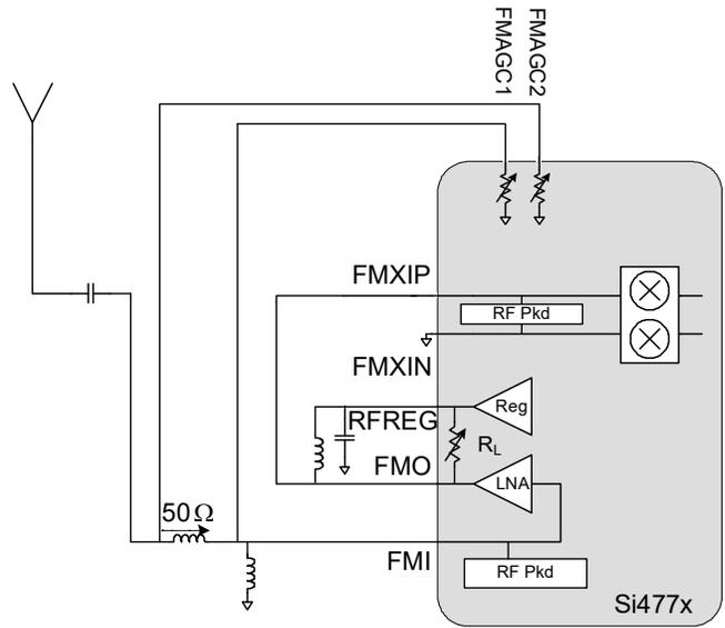
**Figure 10. Conceptual Illustration of the Lowest-Cost Configuration**
