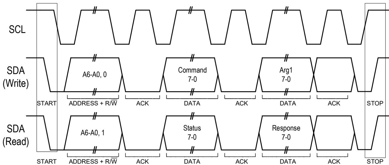
**Figure 4. I<sup>2</sup>C Control Interface Read and Write Timing Diagram**
