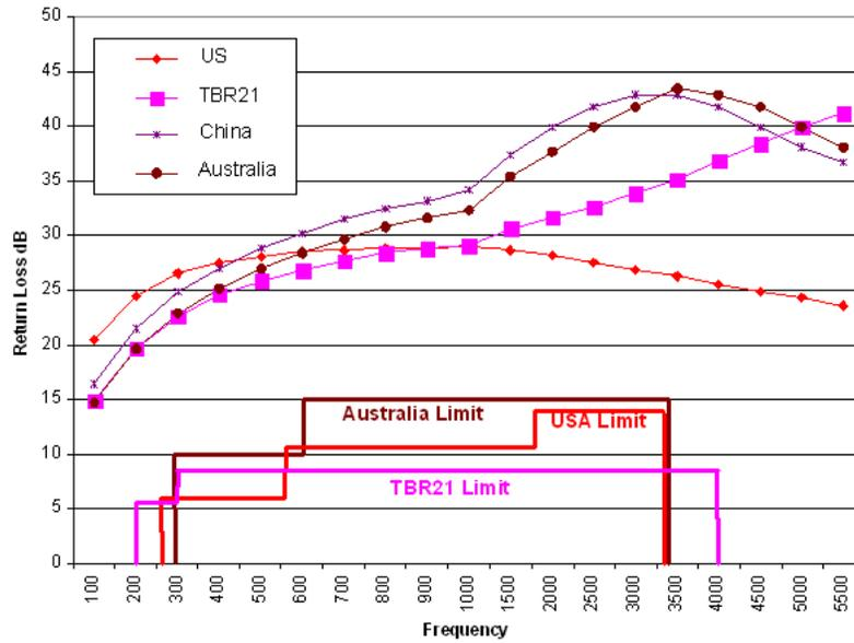
**Figure 1: 73M1x22 Return Loss Characteristics**
