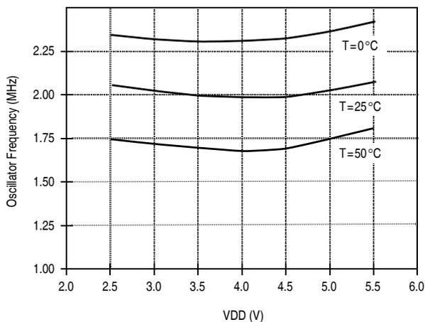
**Figure 2-3** Typical Oscillator Frequency for Wire-Strap Connection
