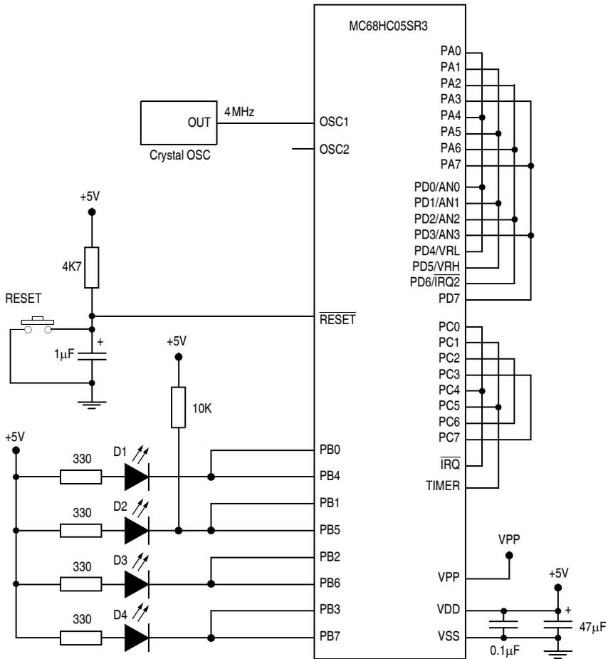
Figure 10-1 MC68HC05SR3 Self-Check Circuit
