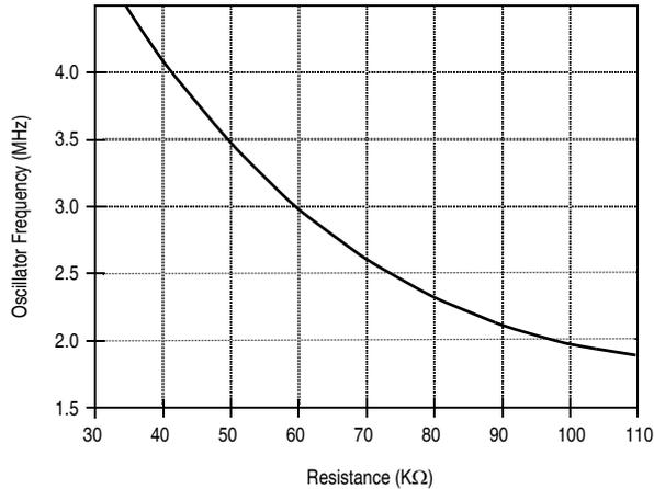
**Figure 2-2** Typical Oscillator Frequency for Selected External Resistor
