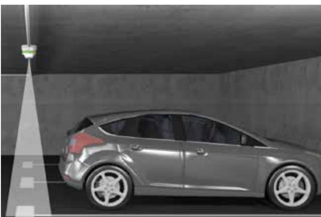
The sensor is wrongly mounted in the lane
