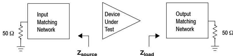
Figure 8. Series Equivalent Source and Load Impedance – 1030–1090 MHz
