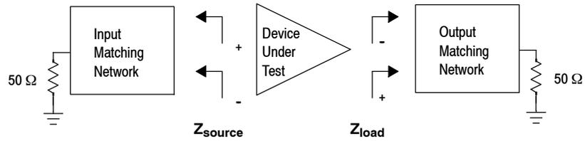
**Figure 15. Series Equivalent Source and Load Impedance – 1030 MHz**
