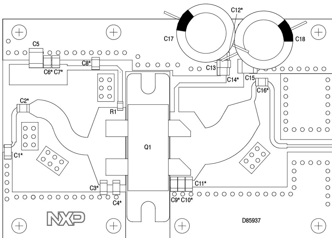
\*C1, C2, C3, C4, C6, C7, C8, C9, C10, C11, C12, C14 and C16 are mounted vertically.
