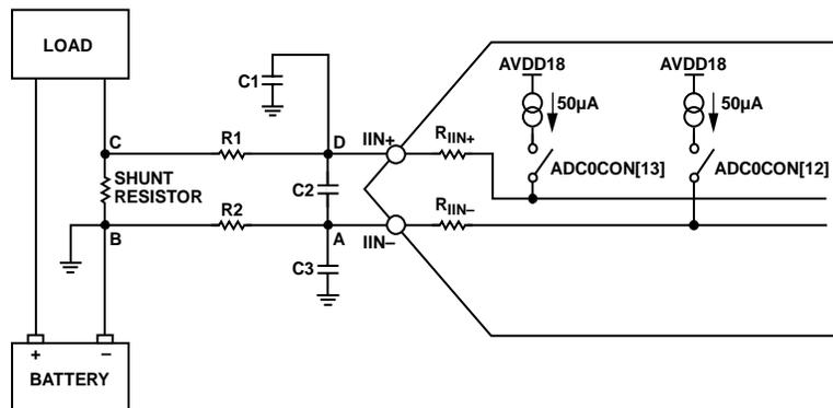
Figure 19. ADC0 Example Circuit Using Diagnostic Current Sources
