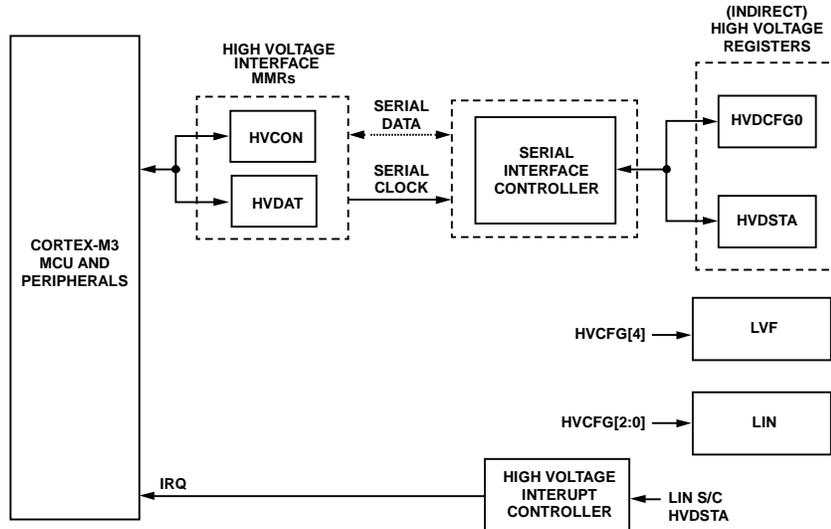
Figure 31. High Voltage Interface, Top-Level Block Diagram
