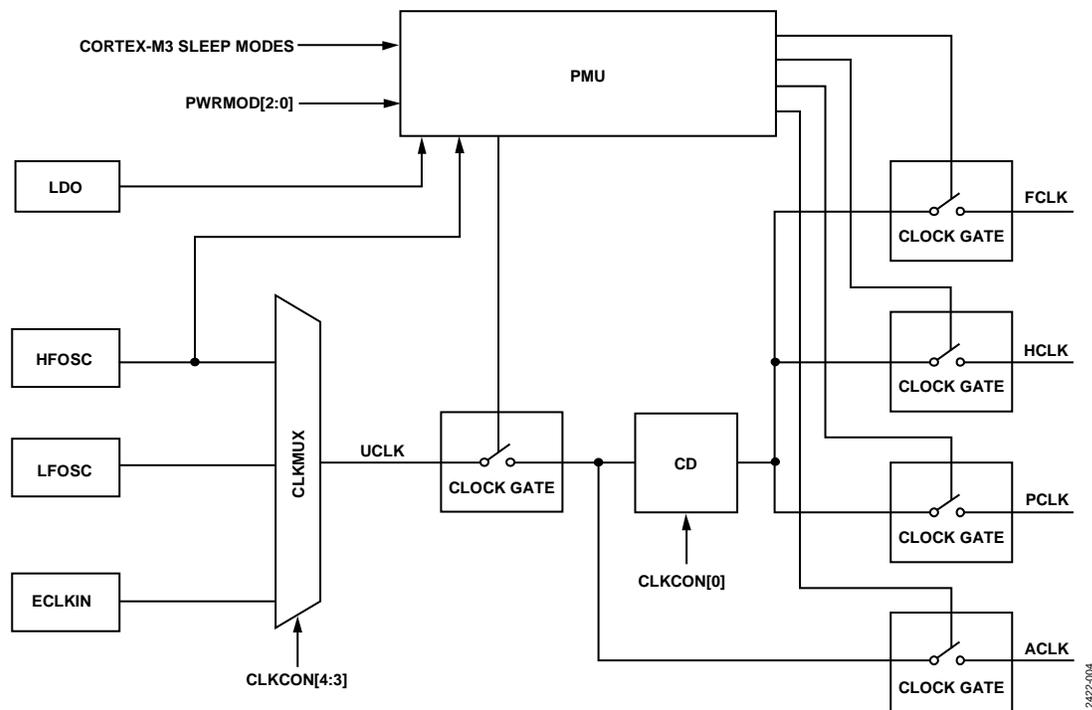
Figure 3. System Clock Architecture Block Diagram
