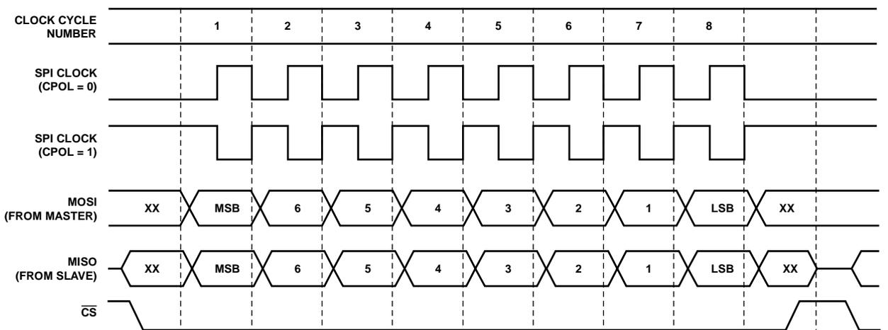
Figure 28. SPI Transfer Protocol, CPHA = 0
