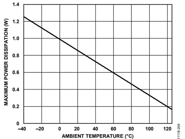
Figure 4. Maximum Power Dissipation vs. Ambient Temperature
