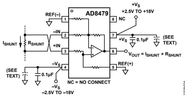
Figure 37. Basic Connections
