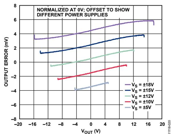
Figure 23. Output Error vs. Output Voltage,  $R_L = 10k\Omega$
