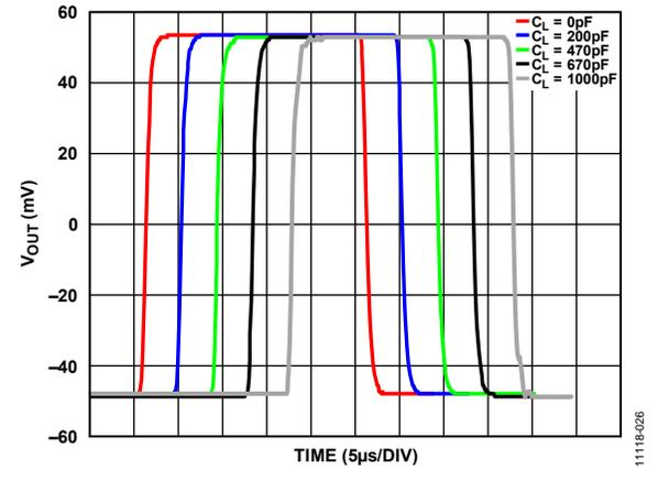
Figure 28. Small Signal Pulse Response vs. Capacitive Load
