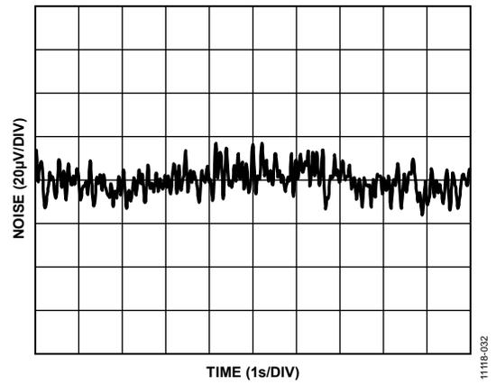
Figure 34. 0.1 Hz to 10 Hz Noise
