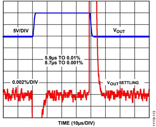
Figure 16. Settling Time
