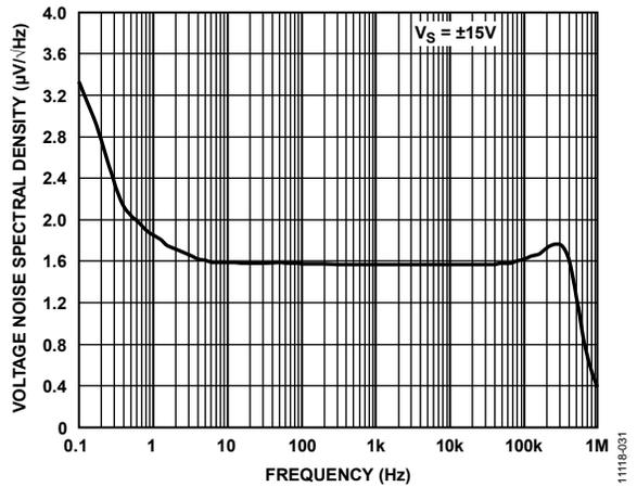
Figure 33. Voltage Noise Spectral Density vs. Frequency
