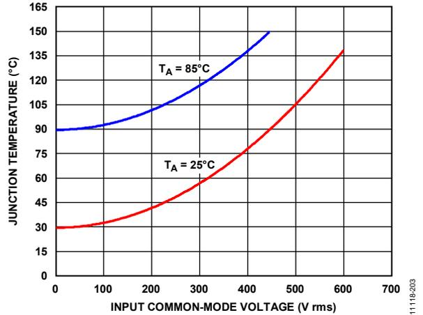
Figure 3. Junction Temperature ( $T_J$ ) vs. Input Common-Mode Voltage
