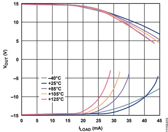
Figure 19. Output Voltage vs. Output Current over Temperature
