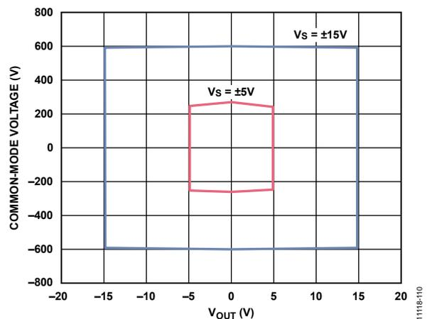
Figure 2. Input Common-Mode Voltage vs. Output Voltage
