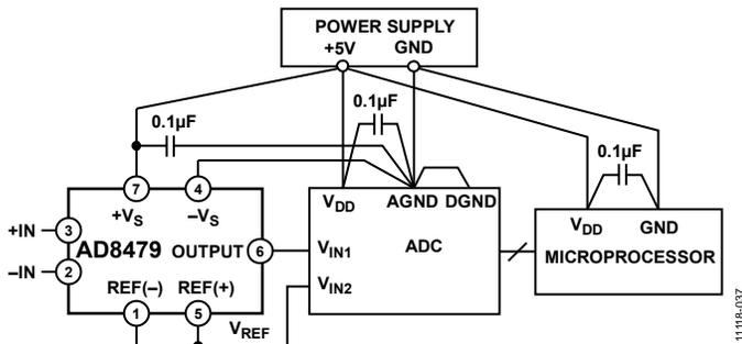
Figure 40. Optimal Grounding Practice for a Single-Supply Environment
