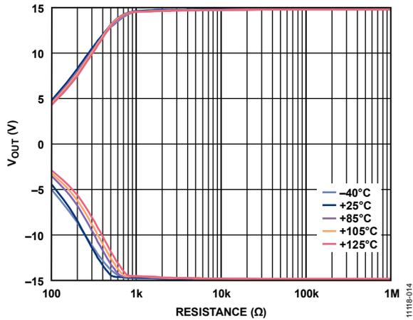
Figure 18. Output Voltage vs. Load over Temperature
