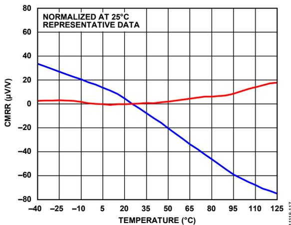
Figure 20. CMRR vs. Temperature,  $V_{CM} = \pm 20V$
