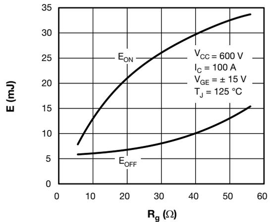
Fig. 4 - IGBT Switching Loss vs.  $R_G$
