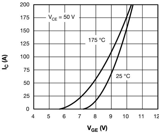
Fig. 2 - IGBT Transfer Characteristics
