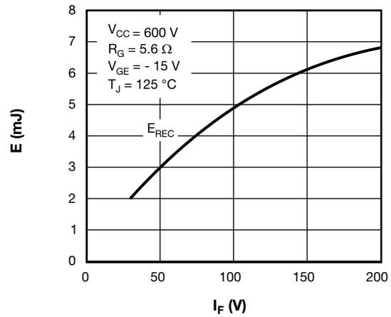
Fig. 8 - Diode Switching Loss vs.  $I_F$
