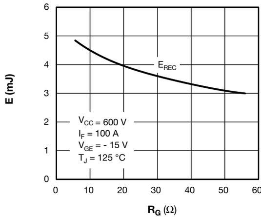
Fig. 9 - Diode Switching Loss vs.  $R_G$
