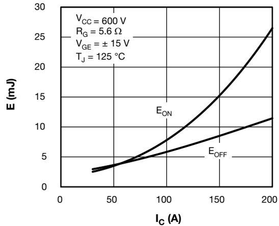
Fig. 3 - IGBT Switching Loss vs.  $I_C$
